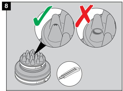
Using a sharp knife pierce a hole in the very end of the nipple you want the cable to run through.
