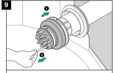
Pull the cables through individual pierced nipples and fit the rubber entry boot back onto the flange. Tighten clips to secure.
