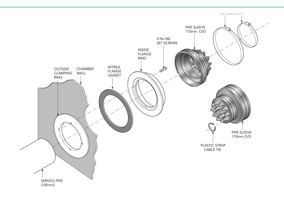
110mm dia. rubber cable entry kit designed to seal up to 16 cables. Supplied with cable ties.
