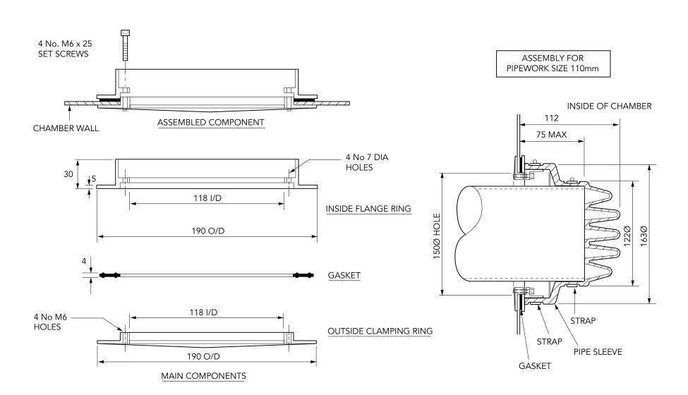
110mm dia. rubber cable entry kit designed to seal up to 16 cables. Supplied with cable ties.
