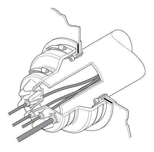
110mm dia. rubber cable entry kit designed to seal up to 16 cables. Supplied with cable ties. For reference purposes only. This drawing is not a specification. Order against product code only. To enable continuous improvement of our products, the designs and specifications are subject to change without notice.
