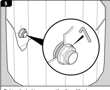
Tighten the locking screw with a 5mm Allen key
