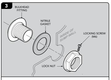
Assemble the electrical cable entry seal as shown ensuring that the gasket is positioned under the flange of the bulkhead fitting on the outside of the sump.
