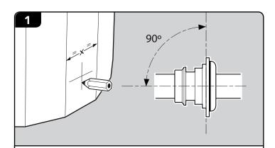
Mark out position for electrical cable entry seal.
