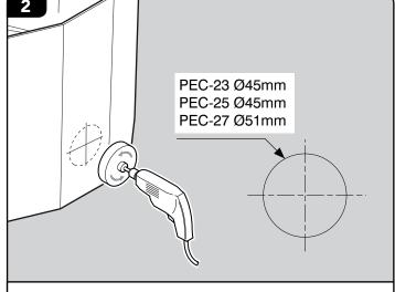
Using a drill piloted 45 mm diameter hole saw cut the correct size hole in the sump wall.
