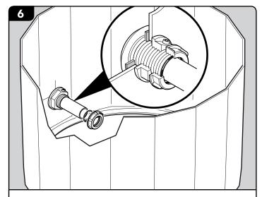
Push the conduit through the electrical cable entry seal and seal the conduit with the 'O' ring and seal nut.
