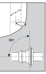
Assemble the electrical cable entry seal as shown ensuring that the gasket is positioned under the flange of the bulkhead fitting on the outside of the sump.
