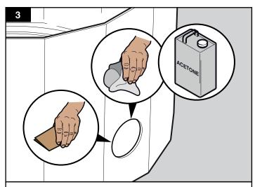
Ensure that the contact area is clean and free from dust and lose material. If necessary clean with sandpaper and Acetone.
