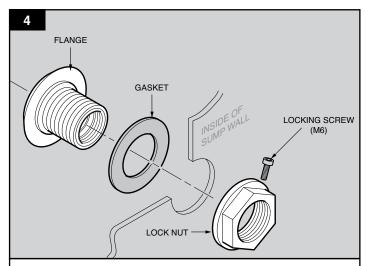
Assemble the electrical cable entry seal ensuring that the gasket is positioned under the flange lip on the outside of the sump.
