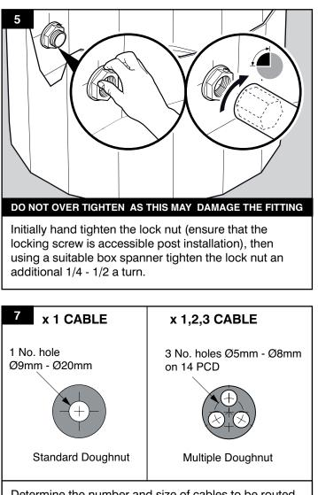
Determine the number and size of cables to be routed through the entry sealkit. Fit the appropriate rubber doughnut (standard or multiple) into the recess of the plastic insert. Ensure there is a washer either side of the doughnut. (standard only).
