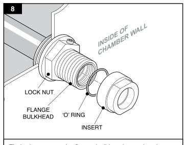
Fit the insert onto the flange bulkhead ensuring that the pre-fitted 'O' ring inside the insert is present before tightening.
