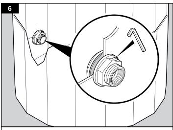
Tighten the locking screw with a 5 mm Allen key
