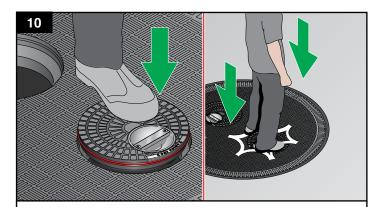
Replace the cover into the parent cover and step on the edges to seat properly. The top edge of the port cover should sit evenly with the top of the parent cover. If port cover does not seat properly, ensure that the interfacing port surfaces are free from residue and that the seal is properly seated in the seal channel.
