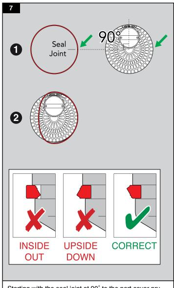
Starting with the seal joint at 90° to the port cover pry point, insert the seal into the cover for approximately 50% of the cover circumference.
