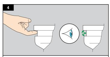
Ensure that the cover seal recess is clean and free from any grit and residue. The seal recess should be smooth and flat to the touch.
