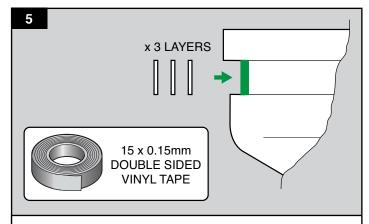
Add 3 layers of  $15 \times 0.15$ mm double sided vinyl tape to the back of the cover groove recess.
