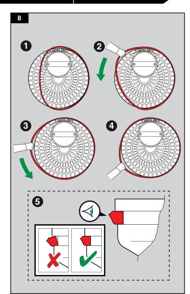
It will be necessary to stretch the remaining length of the seal for it to fit in the cover recess. Visually check to ensure that the seal is correctly fitted.
