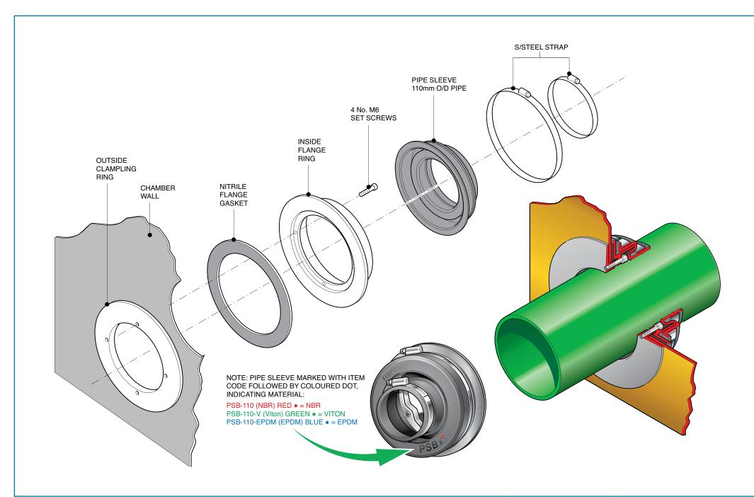
Pipe entry kits to fit 110mm single bore pipework.
