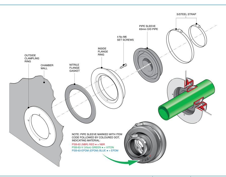
Pipe entry kit to fit 63mm single bore pipework
