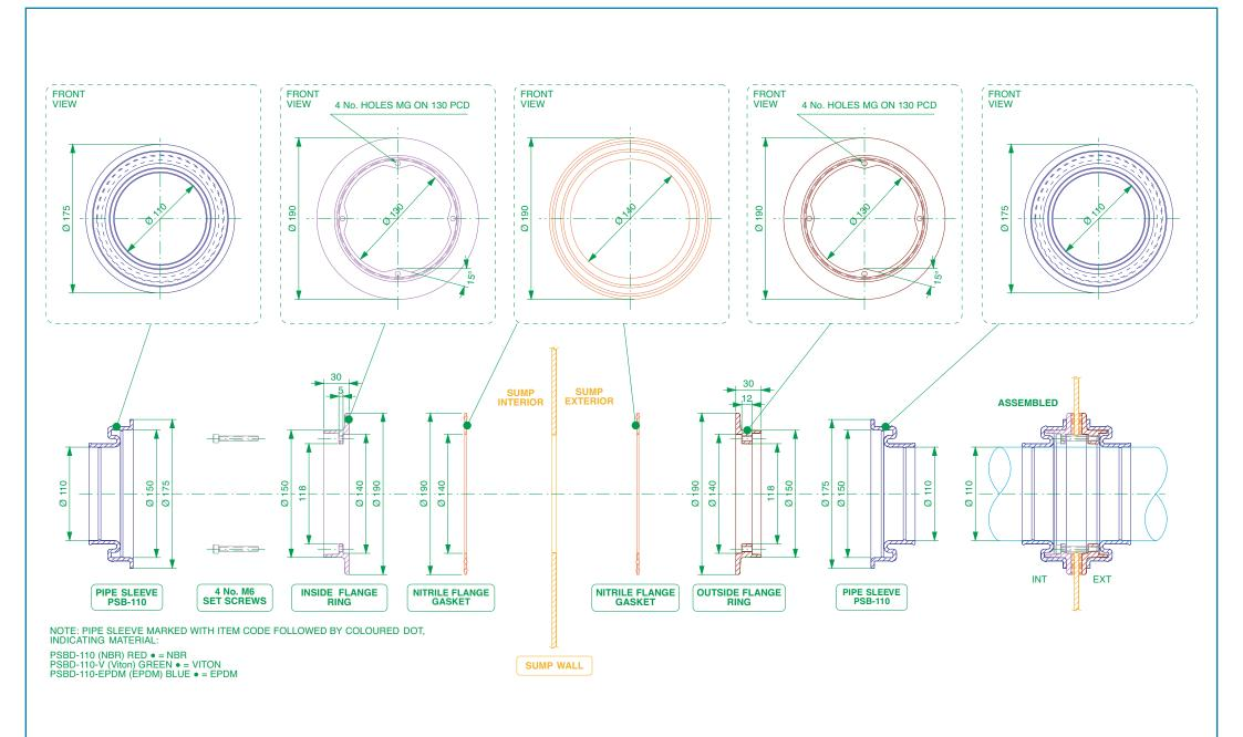
Double sided pipe entry kit to fit 110mm dia. primary pipework
