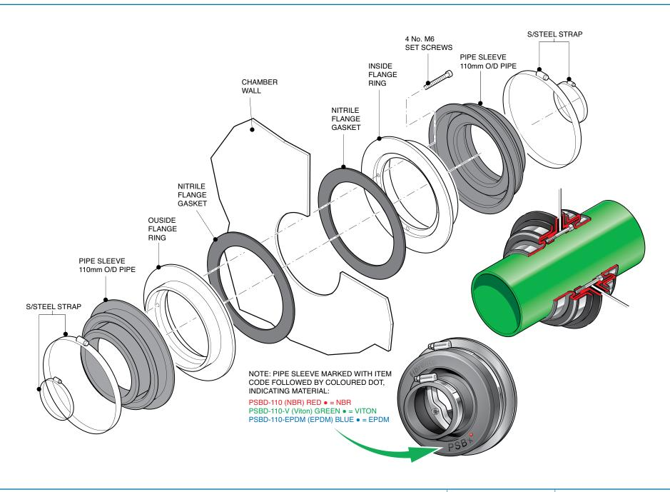
Double sided pipe entry kit to fit 110mm dia. primary pipework
