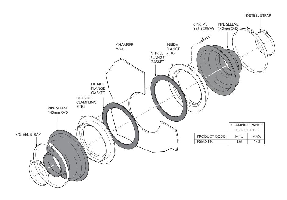
Double sided pipe entry kit to fit 140mm dia. primary pipework.
