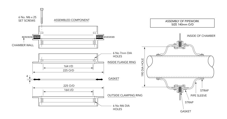
Double sided pipe entry kit to fit 140mm dia. primary pipework.
