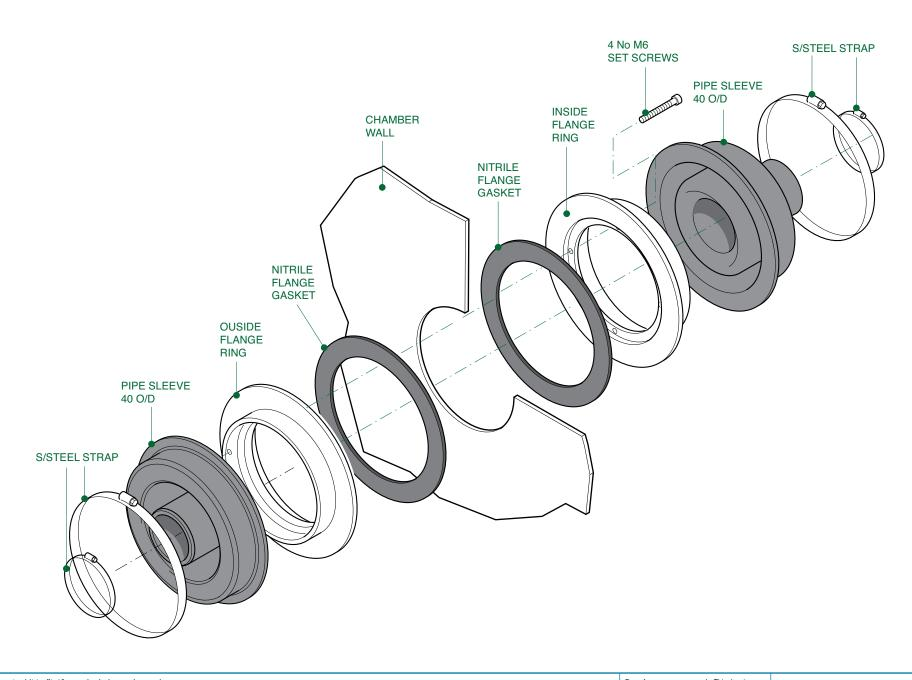
Double sided pipe entry kit to fit 40mm single bore pipework.
