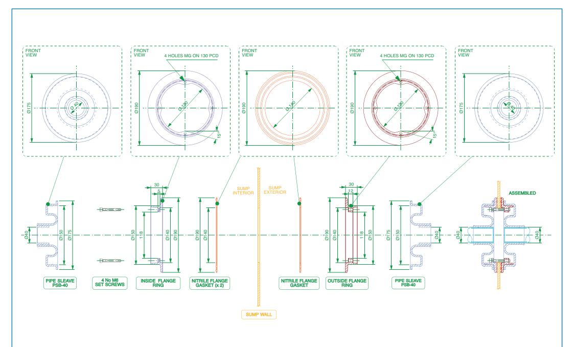
Double sided pipe entry kit to fit 40mm single bore pipework.
