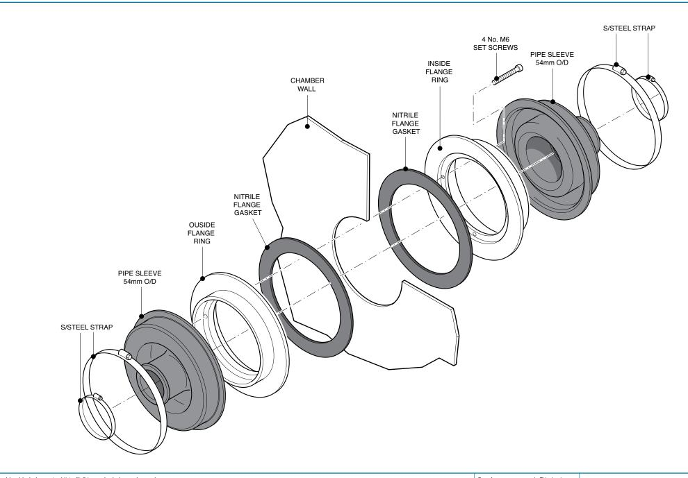
Double sided pipe entry kit to fit 54mm single bore pipework.
