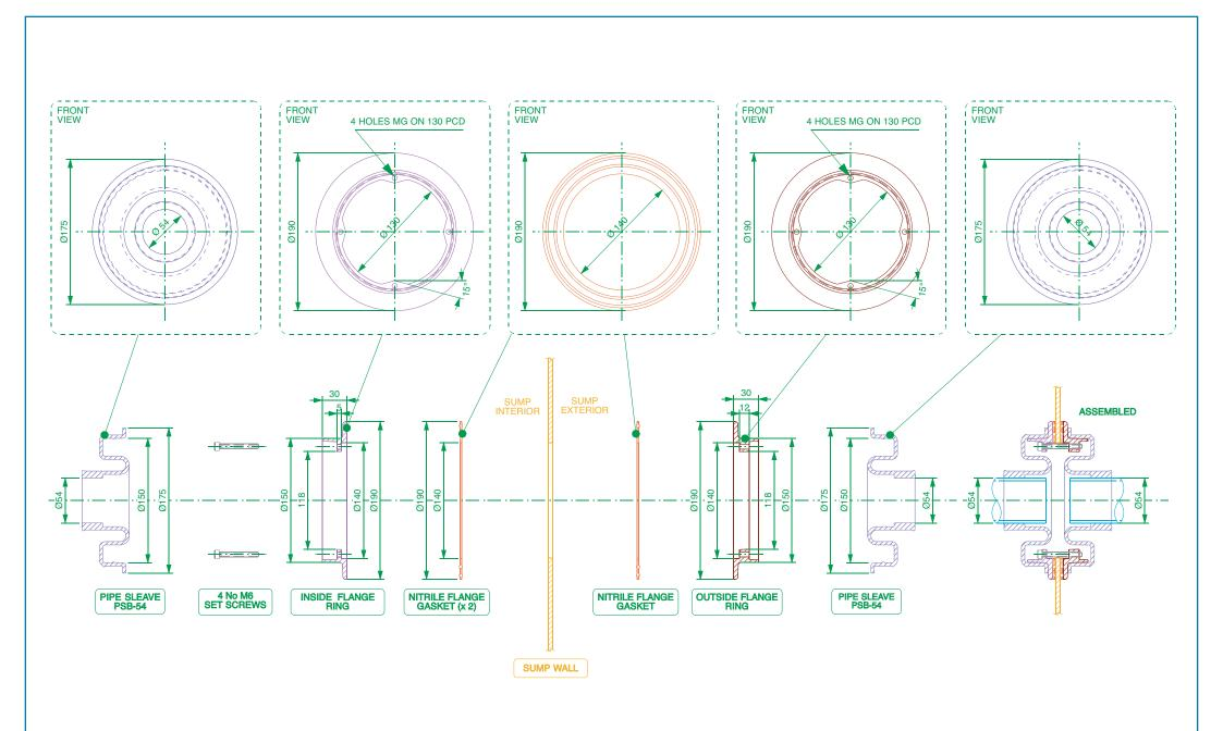
Double sided pipe entry kit to fit 54mm single bore pipework.
