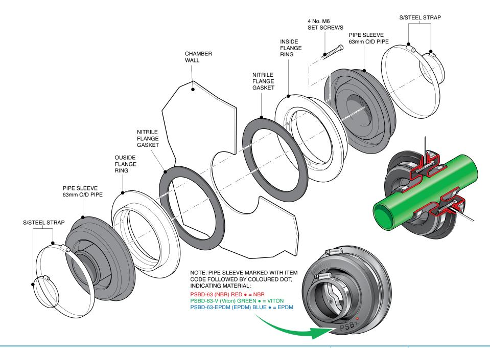
Double sided pipe entry kit to fit 63mm dia. primary pipework
