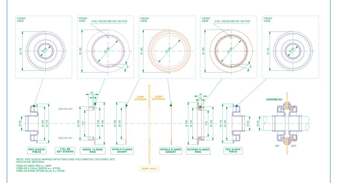
Double sided pipe entry kit to fit 63mm dia. primary pipework
