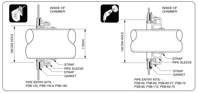
The exit position of the pipework through the chamber wall must be as close as possible to 90°. The pipe kit should be fitted so that the pipework is centrally positioned to the seal. When backfilling ensure that the pipework is not disturbed from this central position.
