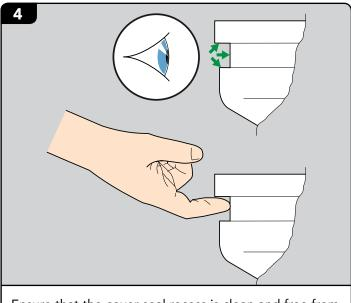
Ensure that the cover seal recess is clean and free from any grit and residue. The seal recess should be smooth and flat to the touch.
