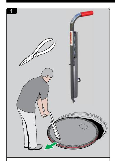
To replace the existing seal, you will require an FL7A lifting handle and a pair of needle nose pliers. To begin, remove the cover from the frame using the FL7A lifting handle.
