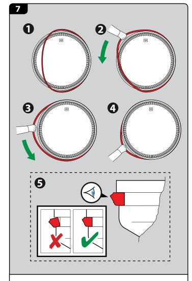
It will be necessary to stretch the remaining length of the seal for it to fit in the cover recess. Visually check to ensure that the seal is correctly fitted.
