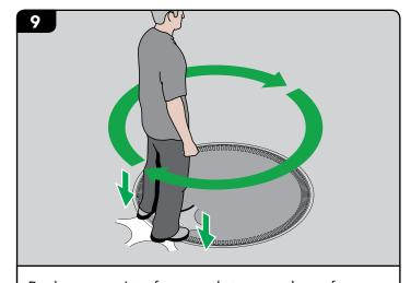
Replace cover into frame and step on edges of cover to seat properly – cover should seat easily into frame so that the top edge of the cover is even with the top of the frame. If cover does not seat properly, ensure that frame is free from residue and that the seal is properly seated in the seal channel.
