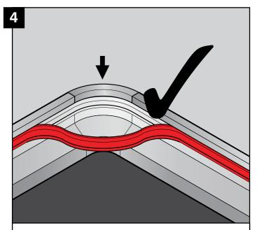
Dry fit the new corner casting to ensure it seats correctly into position and has no obstructions.
