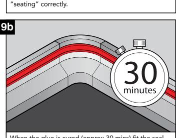
When the glue is cured (approx 30 mins) fit the seal back into the retaining recess.
