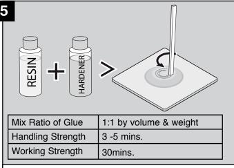
Use chemically resistant goggles/glasses and gloves during mixing and application of the glue. Thoroughly mix a two part glue system resin (R) and hardener (G) in equal amounts onto a suitable board until a uniformed Grey colour is achieved.
