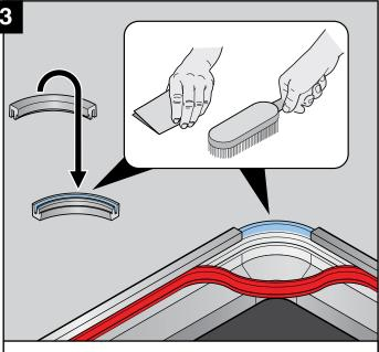
Thoroughly abrade the adhesive contact areas of the corner castings (DO NOT USE SOLVENTS) to remove any debris or glue residue. This can be achieved by using a wire brush or sandpaper. Remove any dust with a clean dry cloth.
