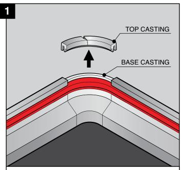
Remove the damaged corner casting. Be careful not to damage the seal as this may effect the covers water tight ability. If the seal is damaged it will need to be removed. Refer to the Seal Replacement Instructions (page 1, steps 1-6) and then continue to step 3.
