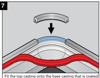
Fit the top casting onto the base casting that is coated with the adhesive.
