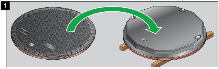
Turn the cover over and elevate using wooden blocks to allow access to the lock paddle and to protect the cover surface.
