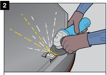
Using a 4" grinder, grind away the weld on the paddle foot.
