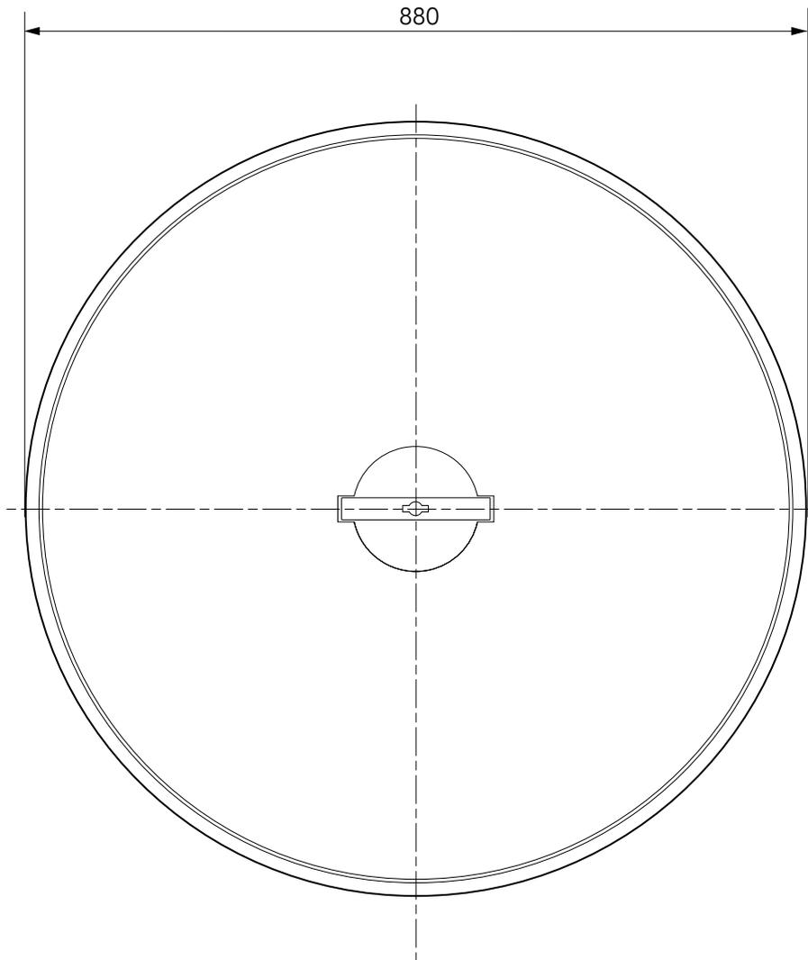
Non-structural standard internal lid to fit all FL90 tank chamber systems.
