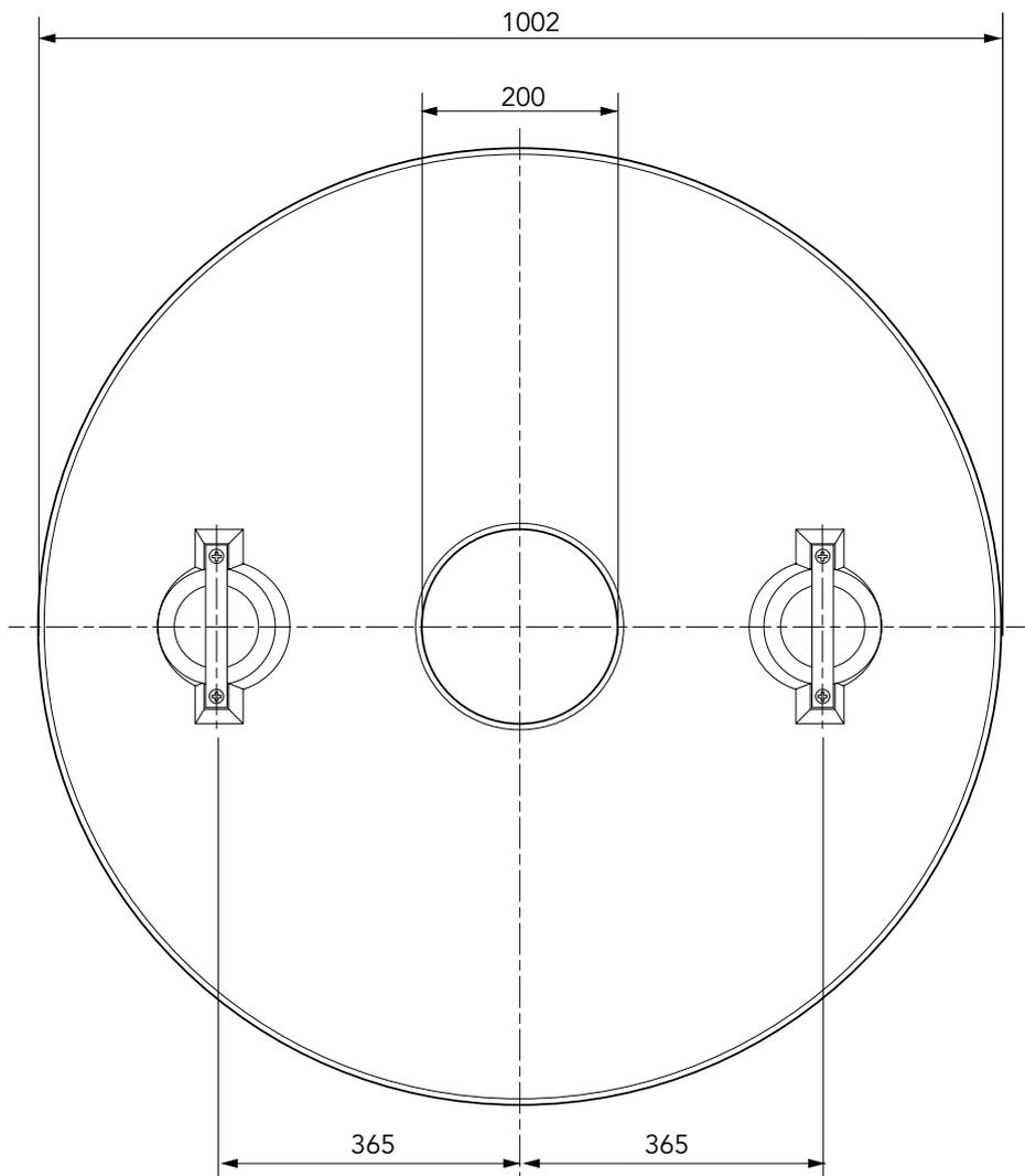
Structural platform with moulded central hole to fit S16-3100/CD & S16CR-3100/CD system. Anti-slip surface.
