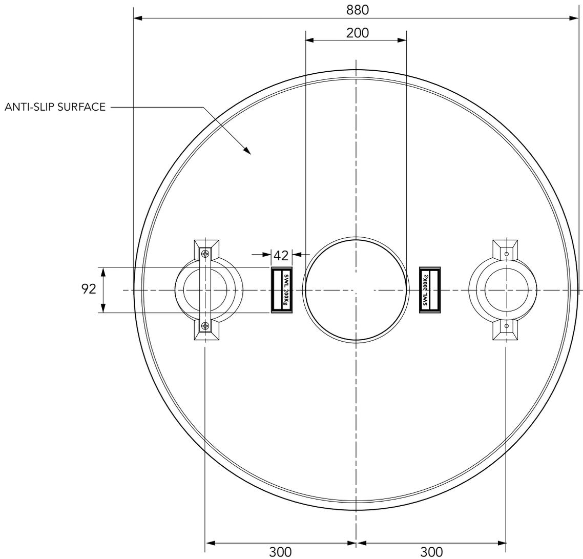
Structural platform with moulded central hole (20cm dia) designed for central fill or dip applications. Fits all chambers systems with FL90 cover. Anti-slip surface.
