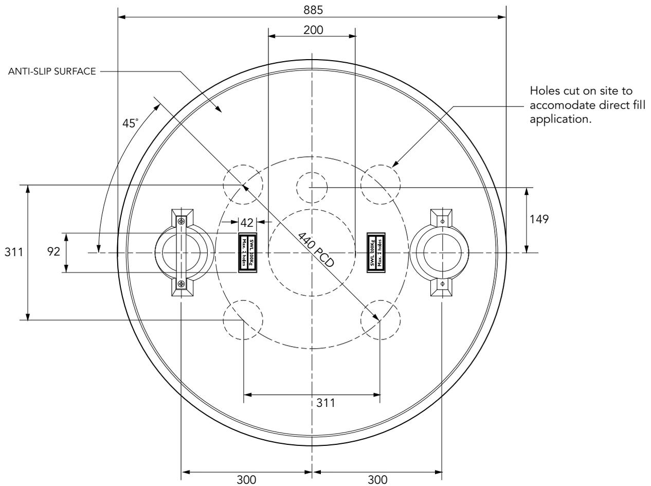
Solid structural platform with hole markings for central fill (20cm dia) and offset dip positions. Fits all chambers systems with FL90 cover. Cut holes on site. Anti-slip surface.
