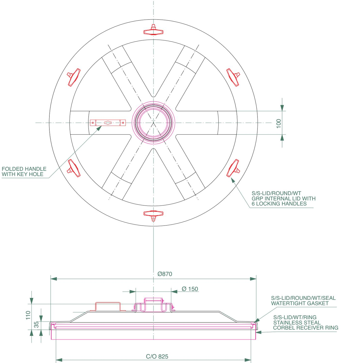
Watertight lock-down internal lid to fit chamber systems with a FL90 cover. Connects to stainless steel corbel ring (S/S-LID/WT/RING).
