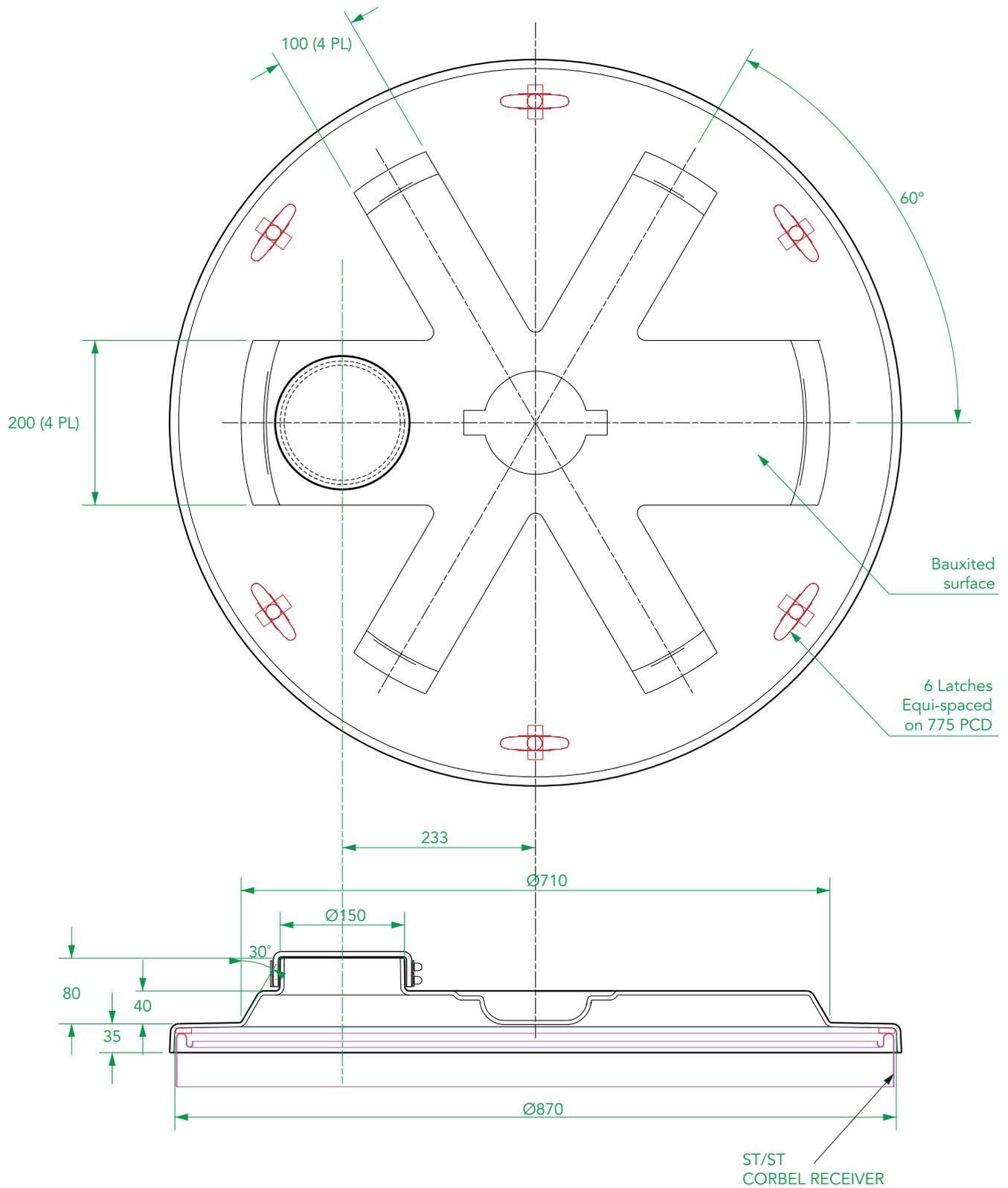
Watertight platform with on offset observation port with 6 locking handles. Fits all chamber systems with FL90 cover or 840mm (33") riser. Includes dip cap. Connects to stainless steel corbel ring.
