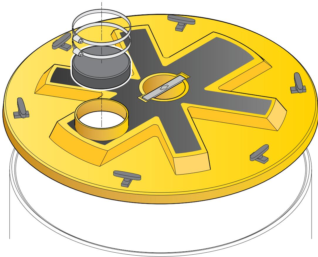
Watertight platform with on offset observation port with 6 locking handles. Fits all chamber systems with FL90 cover or 840mm (33") riser. Includes dip cap. Connects to stainless steel corbel ring.
