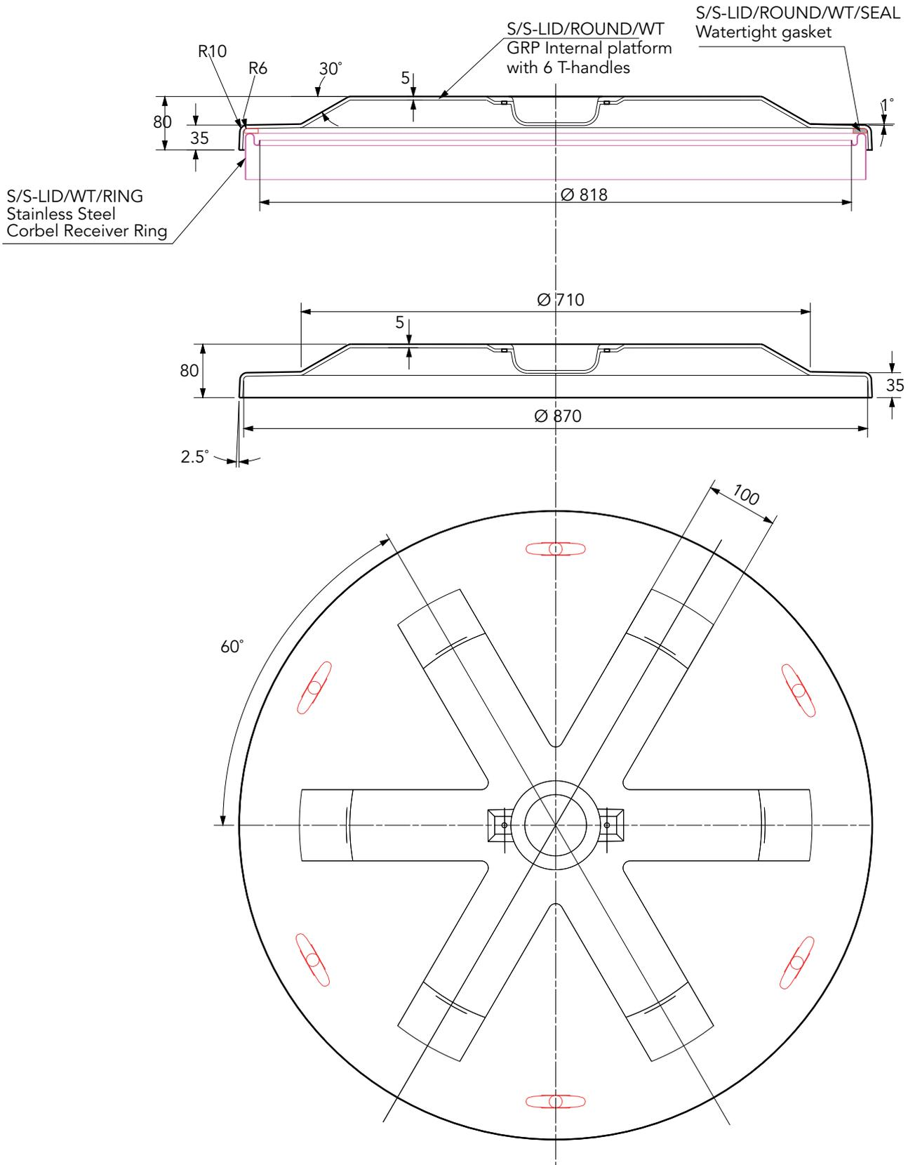
Watertight lock-down internal platform to fit chamber systems with a FL90 cover & 840mm (33") sump riser. Connects to stainless steel corbel ring (S/S-LID/WT/RING)
