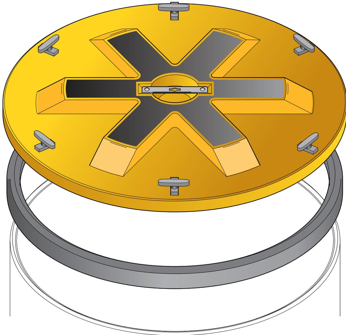
Watertight lock-down internal platform to fit chamber systems with a FL90 cover & 840mm (33") sump riser. Connects to stainless steel corbel ring (S/S-LID/WT/RING)
