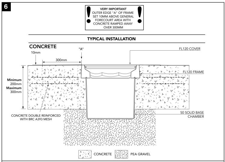
Continue to backfill and concrete. There must be minimum of 200mm and a maximum of 300mm of concrete from grade level. The concrete must be ramped approximately 10mm over 300mm from the edge of frame.
