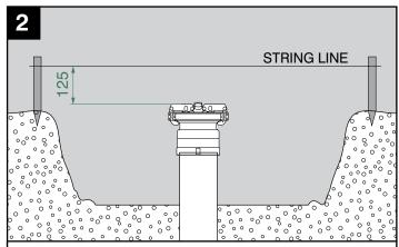
It may be neccesary to trim the riser pipe height. The pipe fitting should sit 125mm from string line.
