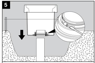
Refit the chamber once the 10mm is acheived and secure the pipekit
