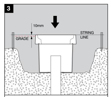
Once the riser is the correct height, fit the chamber and frame. The frame should sit level with the string line which is 10mm above grade level.
