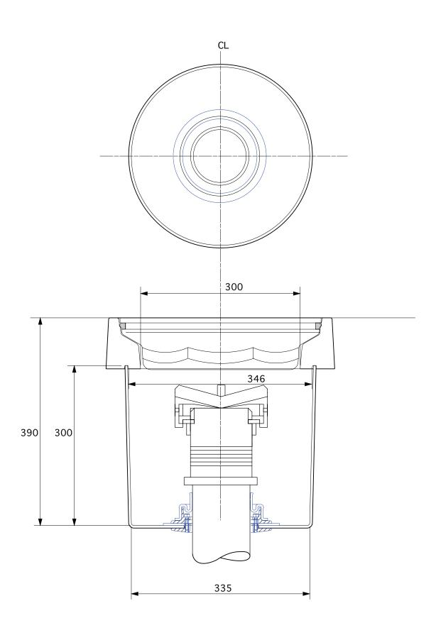
MANUAL DIP GROUNDBOX 300mm dia solid base sump with a 300mm dia grey flat sealed cover and frame. One PSB/110 110mm dia pipe sealkit.
