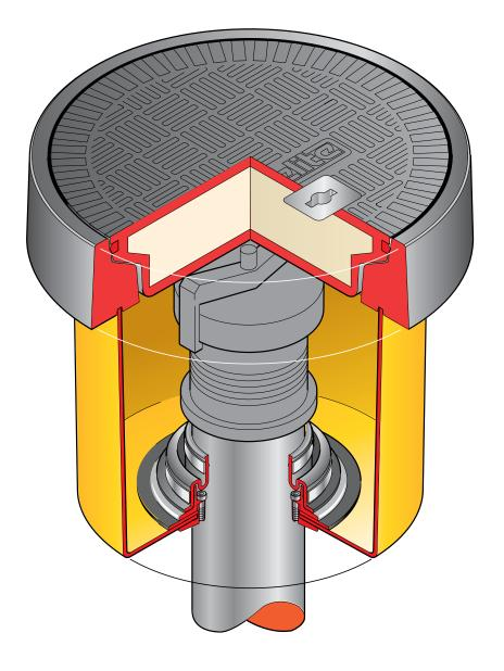
MANUAL DIP GROUNDBOX 300mm dia solid base sump with a 300mm dia grey flat sealed cover and frame. One PSB/110 110mm dia pipe sealkit.
