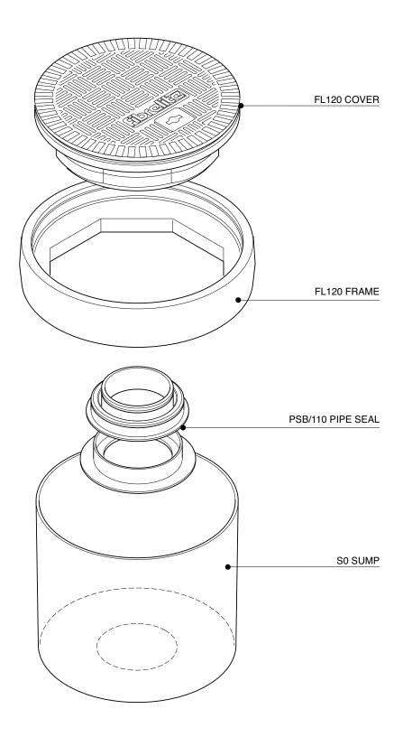
MANUAL DIP GROUNDBOX 300mm dia solid base sump with a 300mm dia grey flat sealed cover and frame. One PSB/110 110mm dia pipe sealkit.
