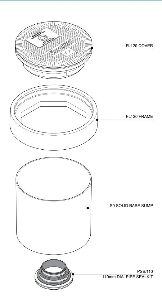
Monitoring Well System. 300mm dia. solid base sump with a 300mm dia. grey flat sealed monitoring well cover with a black ID warning and frame.
