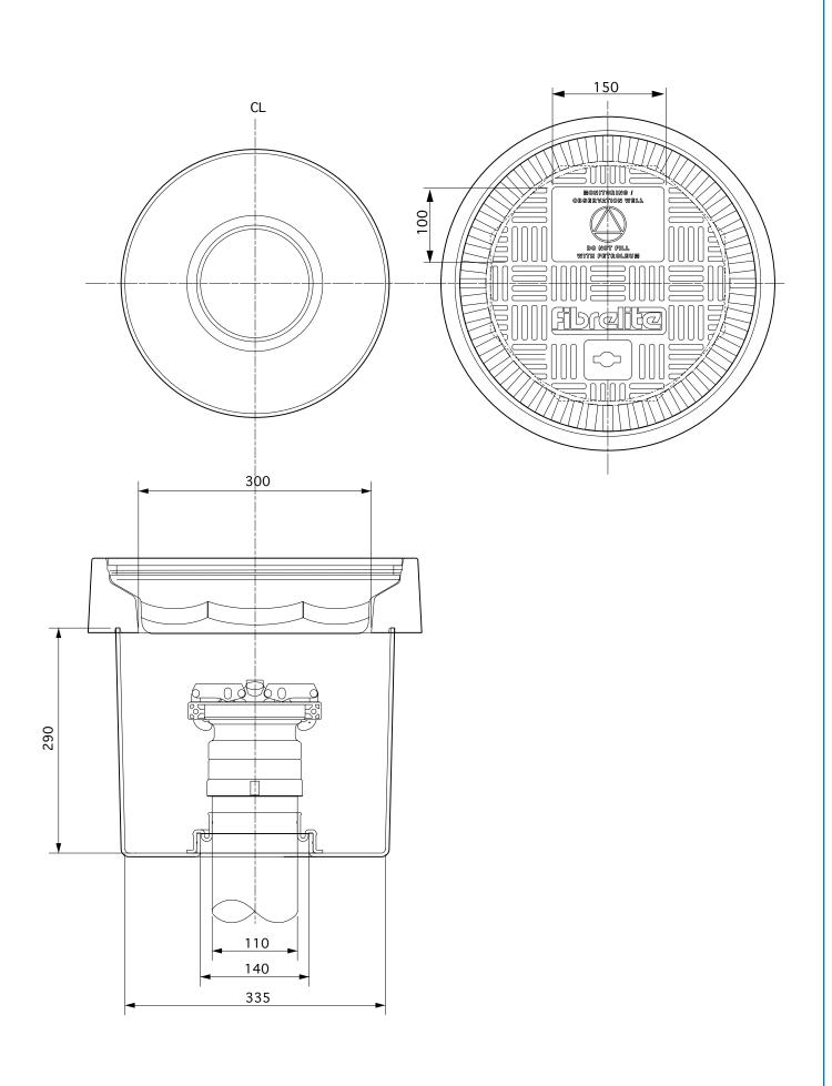
Monitoring Well System. 300mm dia. solid base sump with a 300mm dia. grey flat sealed monitoring well cover with a black ID warning and frame.
