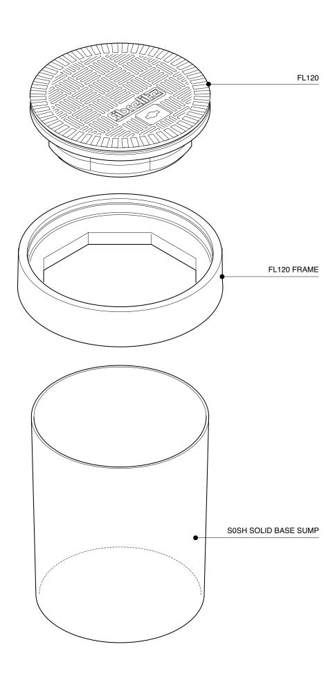
Fixed height 450mm deep, 300mm dia. solid base sump with a 300mm dia. flat sealed cover and frame.
