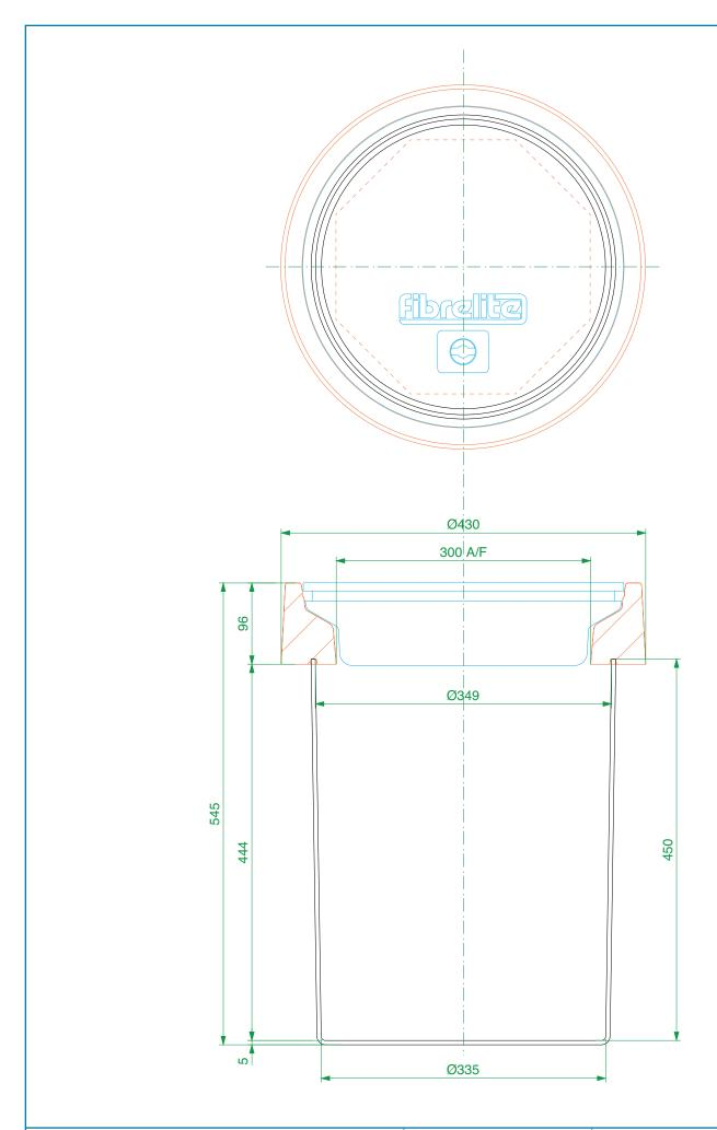
Fixed height 450mm deep, 300mm dia. solid base sump with a 300mm dia. flat sealed cover and frame.
