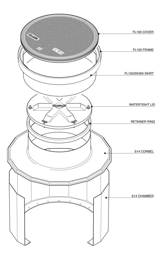
1.4m dia. chamber, sealed corbel with a height adjustable skirt, watertight lid, 1020mm flat sealed cover and frame.
