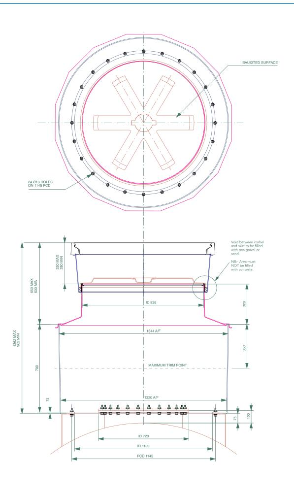
1.4m dia. chamber, sealed corbel with a height adjustable skirt, watertight lid, 1020mm flat sealed cover and frame.
