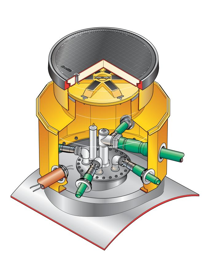
1.4m dia. chamber, sealed corbel with a height adjustable skirt, watertight lid, 1020mm flat sealed cover and frame.
