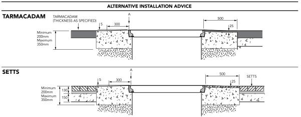
1.4 m dia. chamber, sealed corbel with a height adjustable skirt, watertight lid, 1020mm flat sealed cover and frame.
