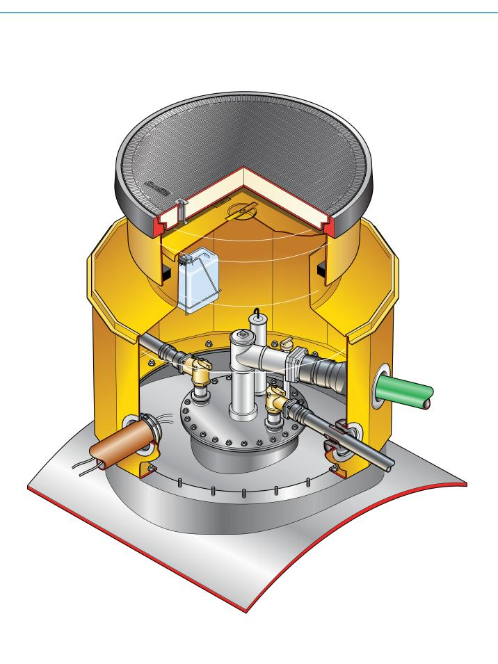
1.4m diameter bolted base chamber, corbel, height adjustable skirt, internal lid, 1020mm dia. watertight flat sealed cover and frame.
