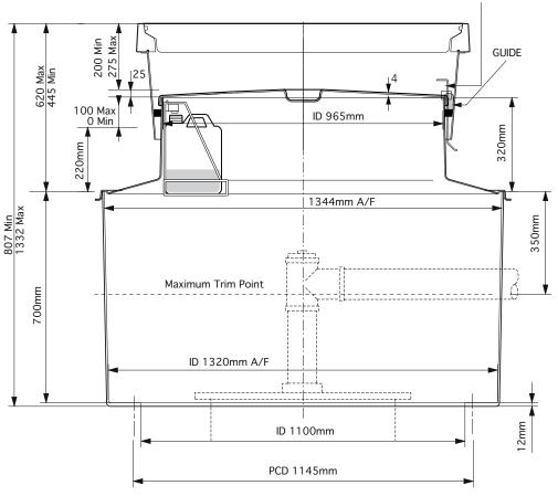
1.4m diameter bolted base chamber, corbel, height adjustable skirt, internal lid, 1020mm dia. watertight flat sealed cover and frame.
