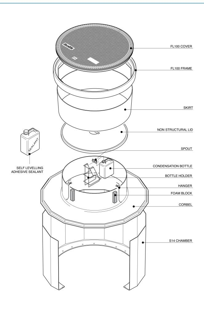
1.4m diameter bolted base chamber, corbel, height adjustable skirt, internal lid, 1020mm dia. watertight flat sealed cover and frame.
