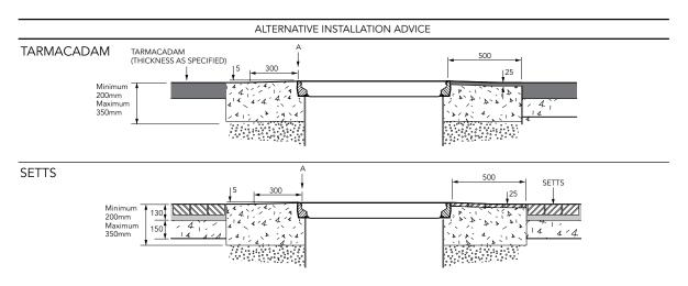
1.4m diameter bolted base chamber, sealed corbel with a height adjustable skirt, non-structural internal lid, round 900mm flat sealed cover with a central port cover and frame. For reference purposes only. This drawing is not a specification. Order against product code only. To enable continuous improvement of our products, the designs and specifications are subject to change without notice.
