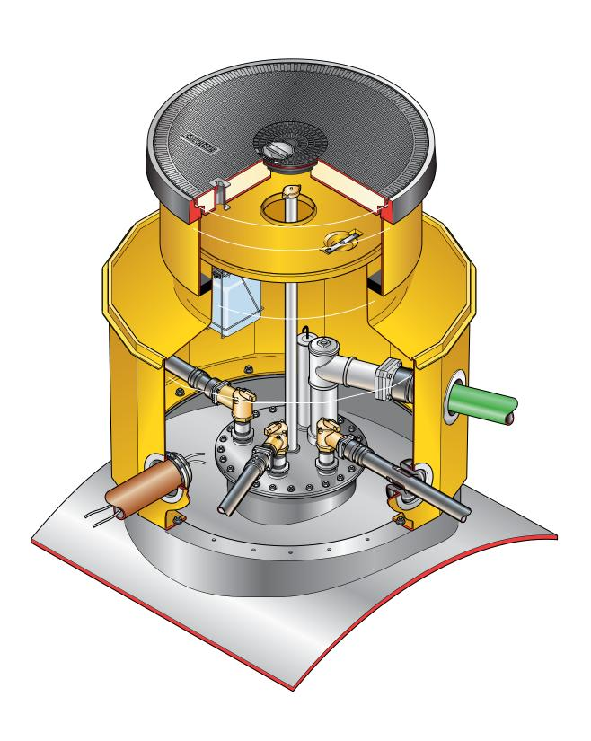
1.4m diameter bolted base chamber, sealed corbel with a height adjustable skirt, non-structural internal lid, round 900mm flat sealed cover with a central port cover and frame.
