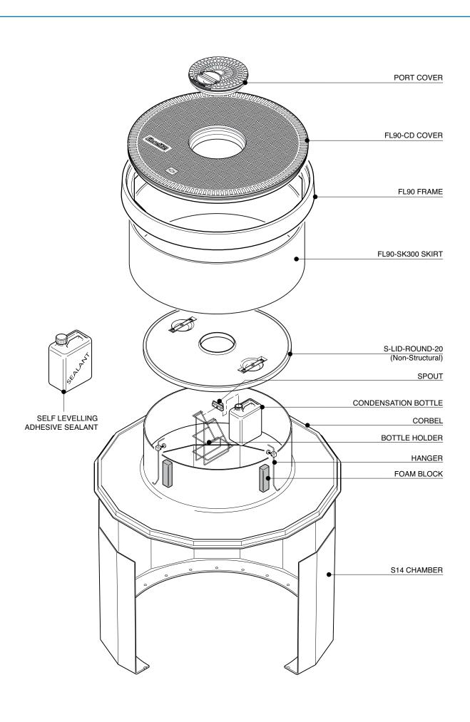
1.4m diameter bolted base chamber, sealed corbel with a height adjustable skirt, non-structural internal lid, round 900mm flat sealed cover with a central port cover and frame.
