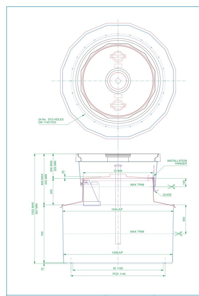
1.4m diameter bolted base chamber, sealed corbel with a height adjustable skirt, non-structural internal lid, round 900mm flat sealed cover with a central port cover and frame.
