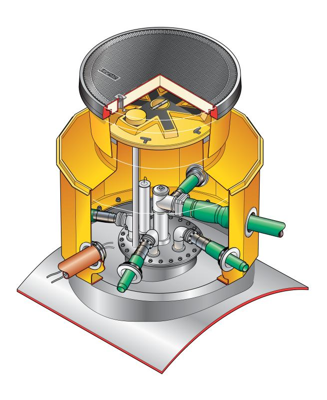
$1.4m\ dia.\ chamber,\ sealed\ corbel\ with\ a\ height\ adjustable\ skirt,\ watertight\ lid,\ 900mm\ flat\ sealed\ cover\ and\ frame.\ Exxon\ Mobil\ European\ Tank\ Chamber.$
