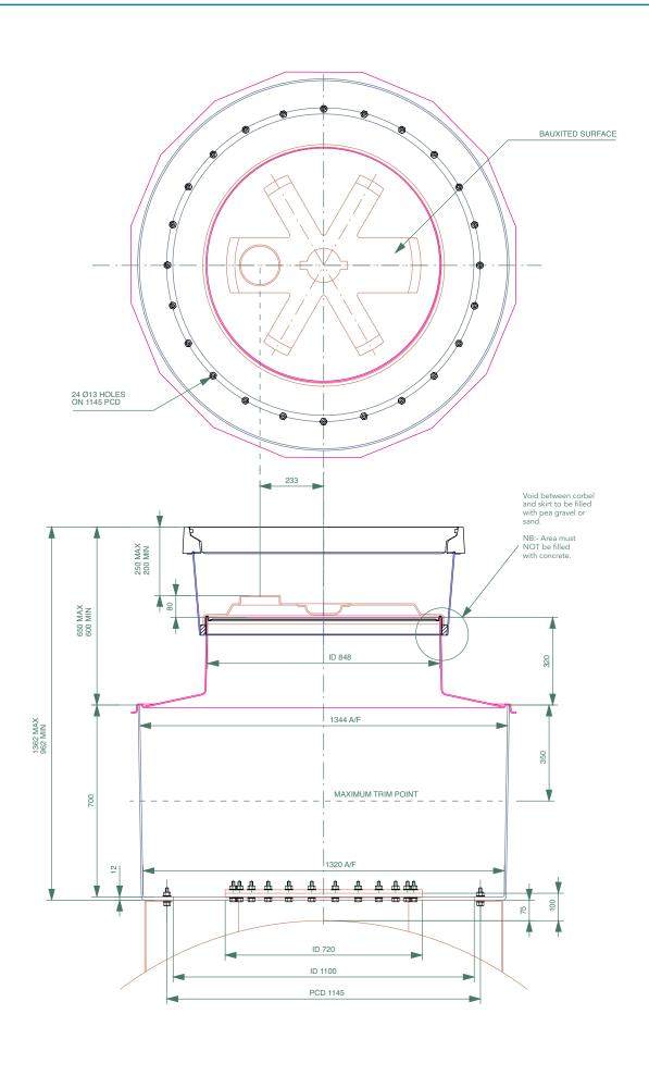
$1.4 m\ dia.\ chamber,\ sealed\ corbel\ with\ a\ height\ adjustable\ skirt,\ watertight\ lid,\ 900mm\ flat\ sealed\ cover\ and\ frame.\ Exxon\ Mobil\ European\ Tank\ Chamber.$
