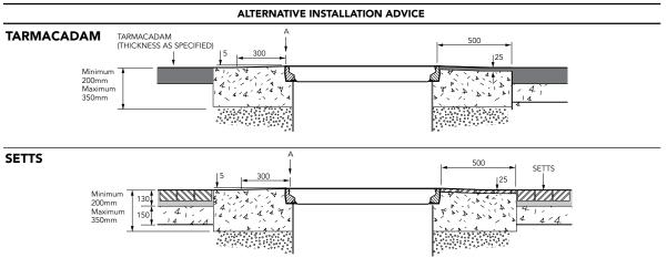
1.4m dia. chamber, sealed corbel with a height adjustable skirt, watertight lid, 900mm flat sealed cover and frame. Exxon Mobil European Tank Chamber.
