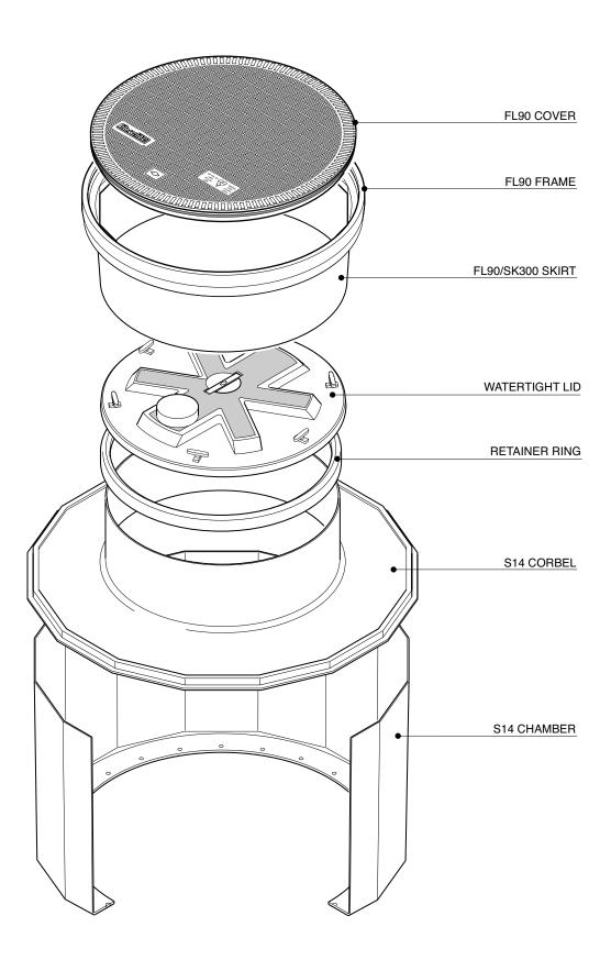
$1.4m\ dia.\ chamber,\ sealed\ corbel\ with\ a\ height\ adjustable\ skirt,\ watertight\ lid,\ 900mm\ flat\ sealed\ cover\ and\ frame.\ Exxon\ Mobil\ European\ Tank\ Chamber.$
