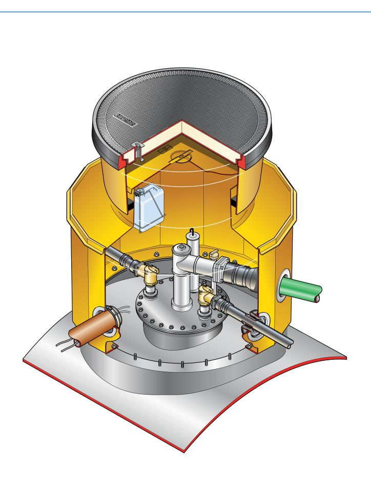
1.4m diameter bolted base chamber, with a corbel, adjustable height skirt, 900mm dia. watertight flat sealed cover and frame.
