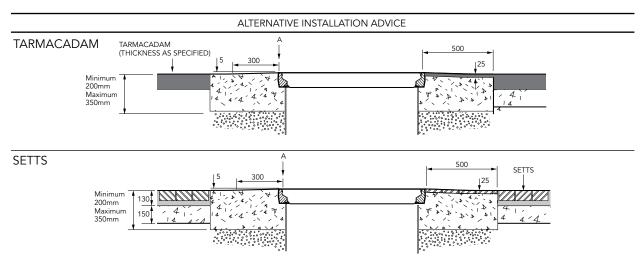
1.4m diameter bolted base chamber, with a corbel, adjustable height skirt, 900mm dia. watertight flat sealed cover and frame.
