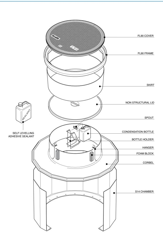
1.4m diameter bolted base chamber, with a corbel, adjustable height skirt, 900mm dia. watertight flat sealed cover and frame.
