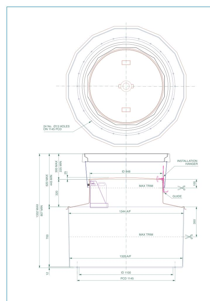
1.4m diameter bolted base chamber, with a corbel, adjustable height skirt, 900mm dia. watertight flat sealed cover and frame.
