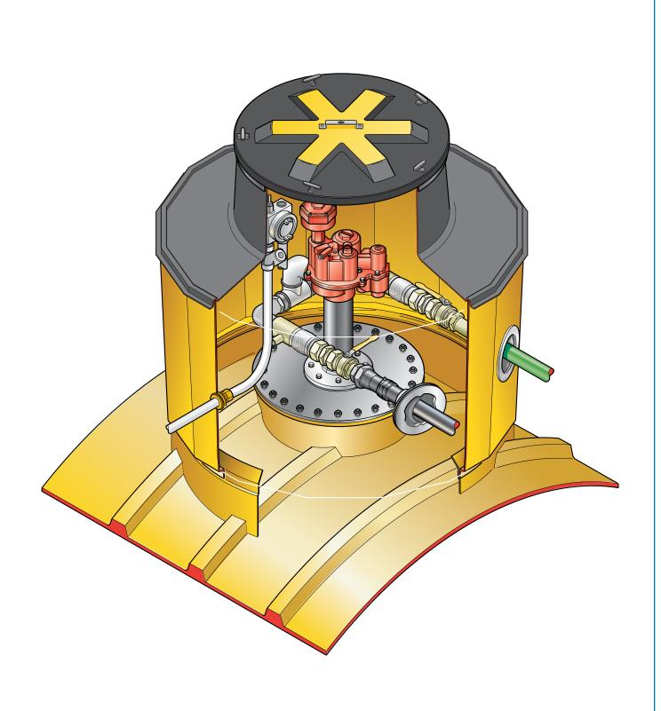
1.4m diameter sump with collar ring base, corbel and watertight platform for green areas.
