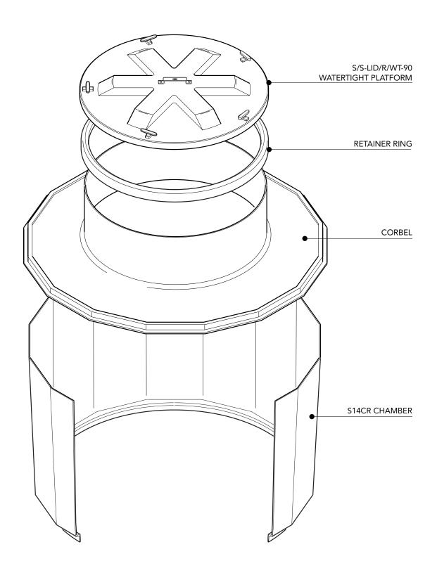
$1.4\mbox{m}$  diameter sump with collar ring base, corbel and watertight platform for green areas.
