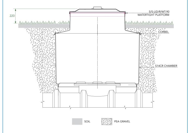
$1.4\mbox{m}$  diameter sump with collar ring base, corbel and watertight platform for green areas.
