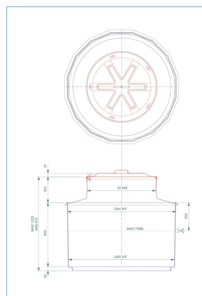
$1.4\mbox{m}$  diameter sump with collar ring base, corbel and watertight platform for green areas.
