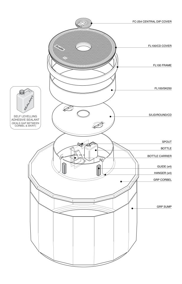
$1.4m\ diameter\ sump\ with\ collar\ ring\ base,\ corbel,\ skirt,\ non-structural\ internal\ lid\ with\ moulded\ hole,\ round\ 1020mm\ flat\ sealed\ central\ dip\ cover.$
