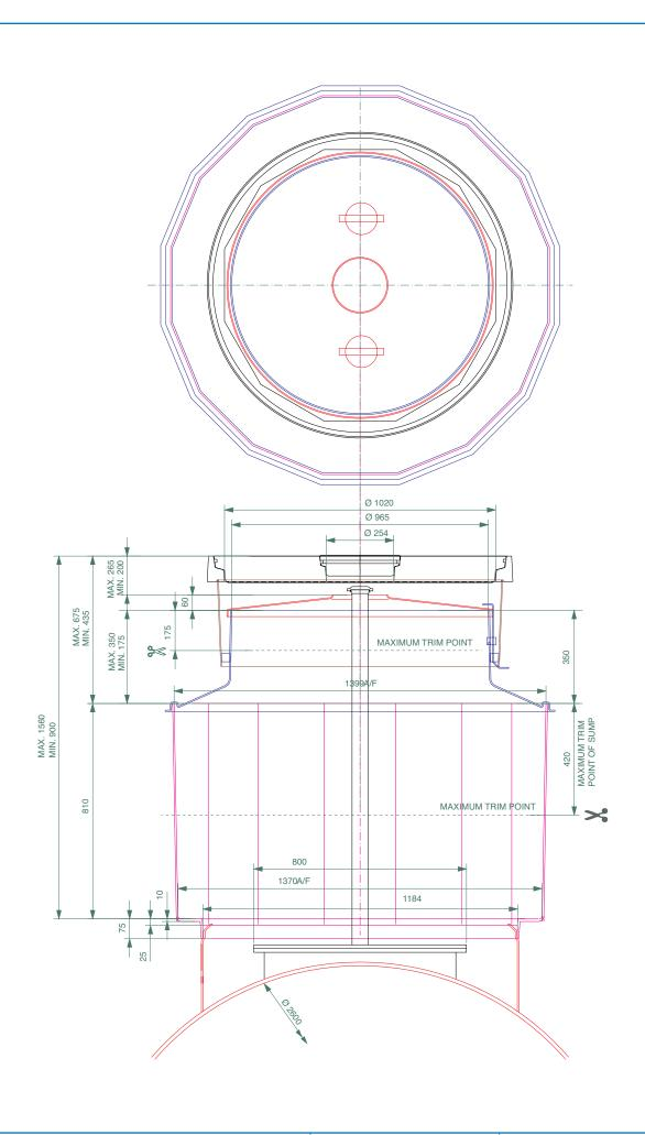
1.4m diameter sump with collar ring base, corbel, skirt, non-structural internal lid with moulded hole, round 1020mm flat sealed central dip cover.
