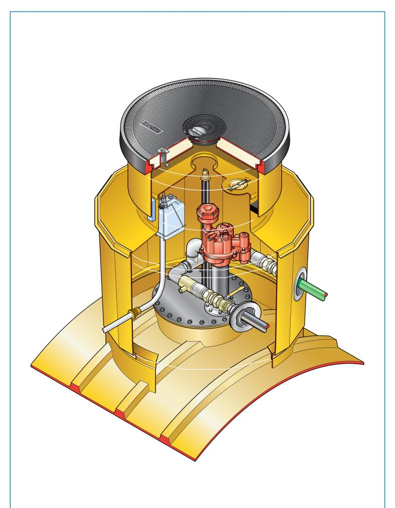
1.4m diameter sump with collar ring base, corbel, skirt, non-structural internal lid with moulded hole, round 1020mm flat sealed central dip cover.
