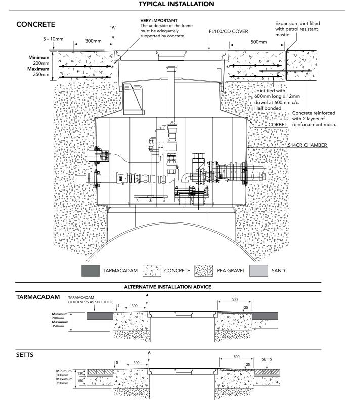
1.4m diameter sump with collar ring base, corbel, skirt, non-structural internal lid with moulded hole, round 1020mm flat sealed central dip cover.
