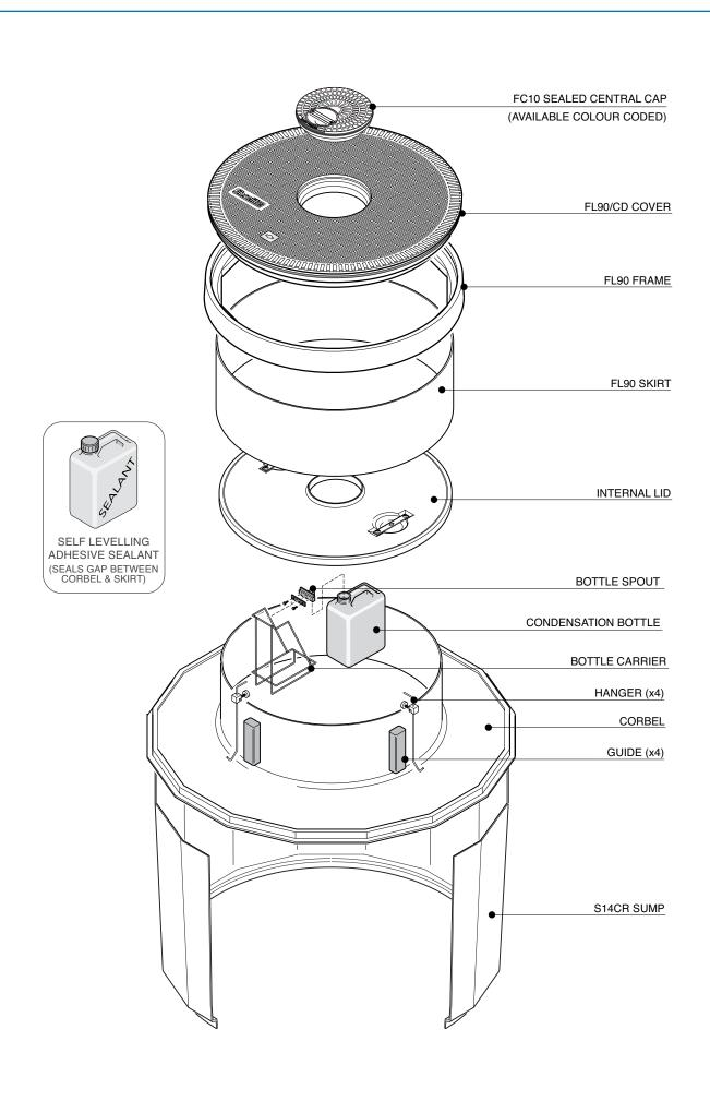
1.2m diameter sump to fit 1.2m collar ring, with corbel, internal lid, adjustable skirt and round 900mm flat sealed cover, corbel/skirt sealkit with condensation bottle and fixing kit.
