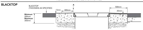
1.2m diameter sump to fit 1.2m collar ring, with corbel, internal lid, adjustable skirt and round 900mm flat sealed cover, corbel/skirt sealkit with condensation bottle and fixing kit.
