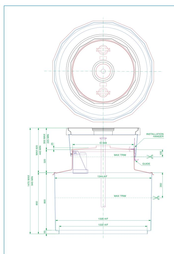
1.2m diameter sump to fit 1.2m collar ring, with corbel, internal lid, adjustable skirt and round 900mm flat sealed cover, corbel/skirt sealkit with condensation bottle and fixing kit.
