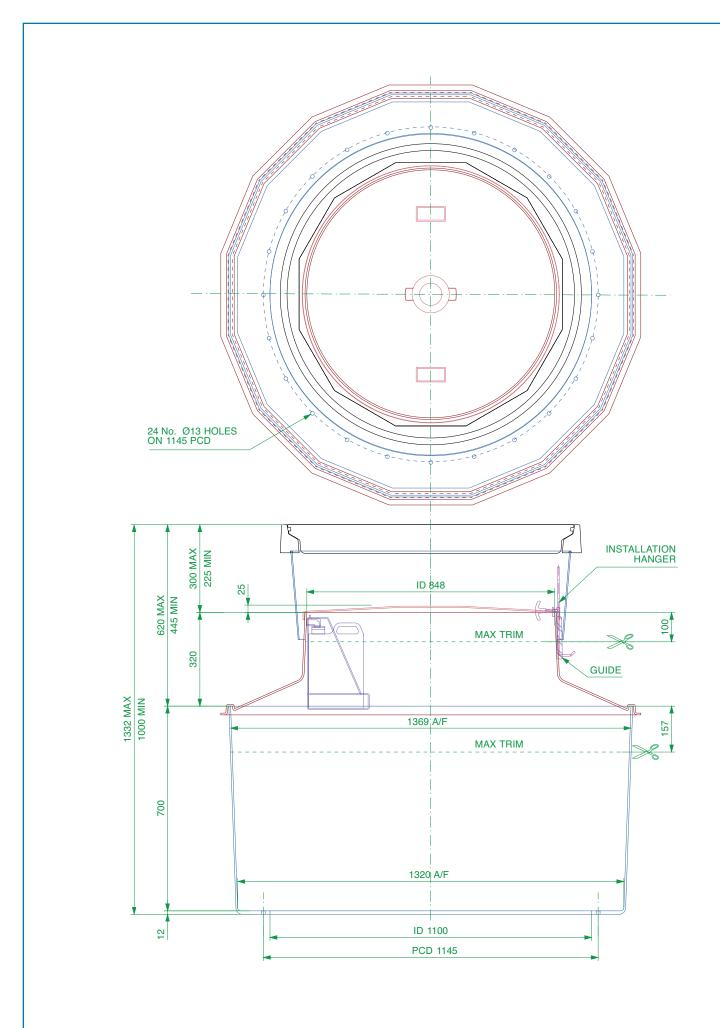
1.4m diameter stackable bolted base chamber, corbel, non-structural internal lid, adjustable height skirt, 900mm diameter watertight flat sealed cover and frame.
