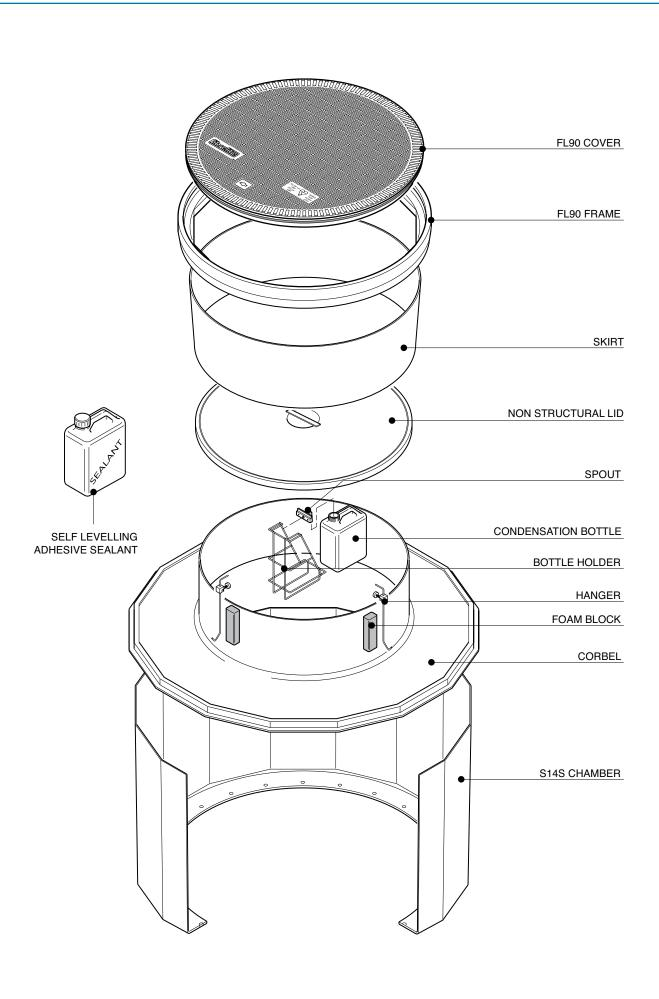
$1.4m\ diameter\ stackable\ bolted\ base\ chamber,\ corbel,\ non-structural\ internal\ lid,\ adjustable\ height\ skirt,\ 900mm\ diameter\ watertight\ flat\ sealed\ cover\ and\ frame.$
