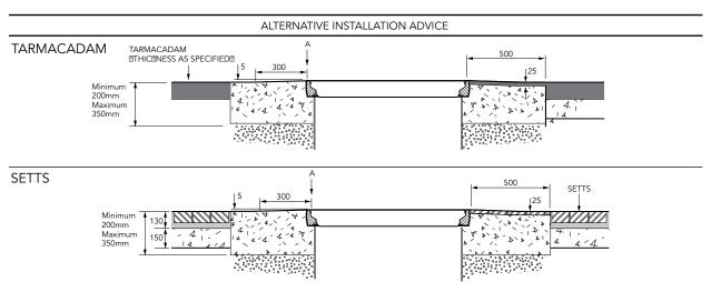
1.4m diameter stackable bolted base chamber, corbel, non-structural internal lid, adjustable height skirt, 900mm diameter watertight flat sealed cover and frame.
