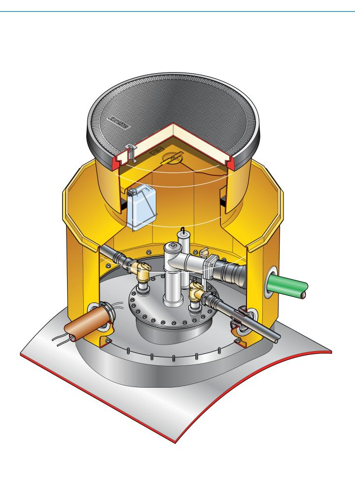
1.4m diameter stackable bolted base chamber, corbel, non-structural internal lid, adjustable height skirt, 900mm diameter watertight flat sealed cover and frame.
