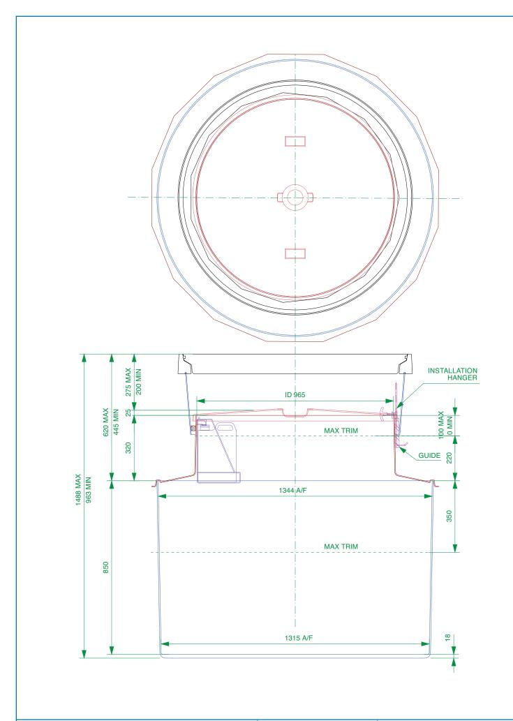
1.4m diameter solid bolted base chamber, with a corbel, adjustable height skirt, 1020mm dia. watertight flat sealed cover and frame.
