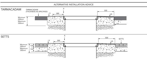
1.4m diameter solid bolted base chamber, with a corbel, adjustable height skirt, 1020mm dia. watertight flat sealed cover and frame.
