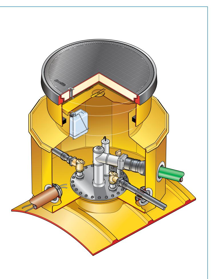
1.4m diameter solid bolted base chamber, with a corbel, adjustable height skirt, 1020mm dia. watertight flat sealed cover and frame.
