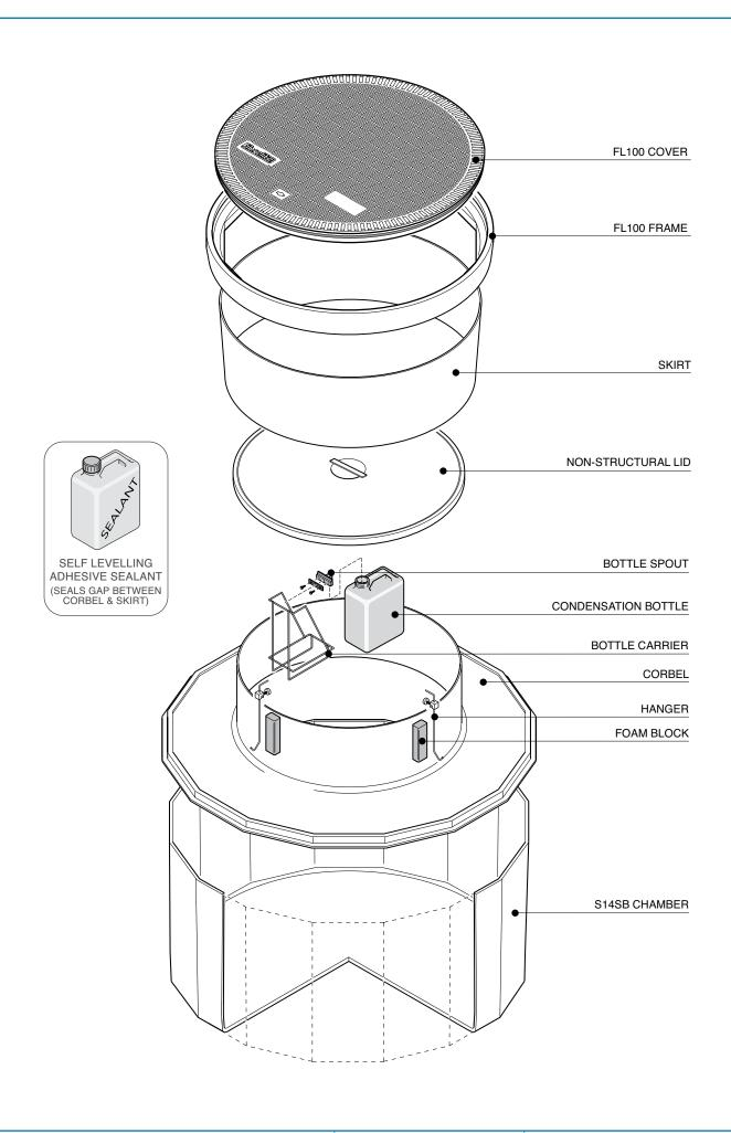
1.4m diameter solid bolted base chamber, with a corbel, adjustable height skirt, 1020mm dia. watertight flat sealed cover and frame.
