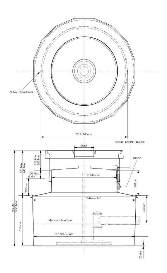
1.4m dia. chamber, corbel with a height adjustable skirt, non-structural internal lid, hand cap and round 900mm flat sealed cover with a central manual dip cover.
