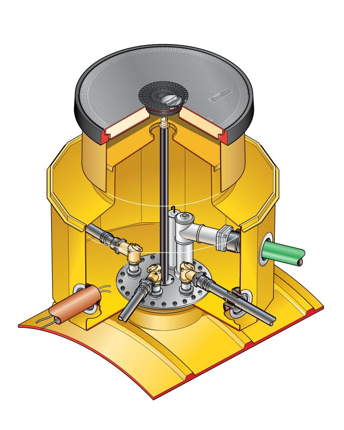
1.4m dia. chamber, corbel with a height adjustable skirt, non-structural internal lid, hand cap and round 900mm flat sealed cover with a central manual dip cover.
