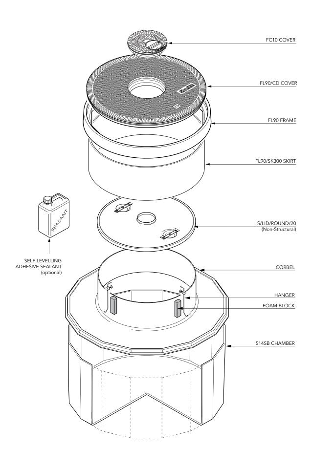
1.4m dia. chamber, corbel with a height adjustable skirt, non-structural internal lid, hand cap and round 900mm flat sealed cover with a central manual dip cover.
