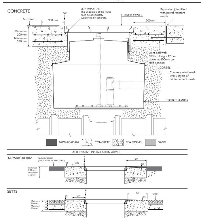
1.4m dia. chamber, corbel with a height adjustable skirt, non-structural internal lid, hand cap and round 900mm flat sealed cover with a central manual dip cover.
