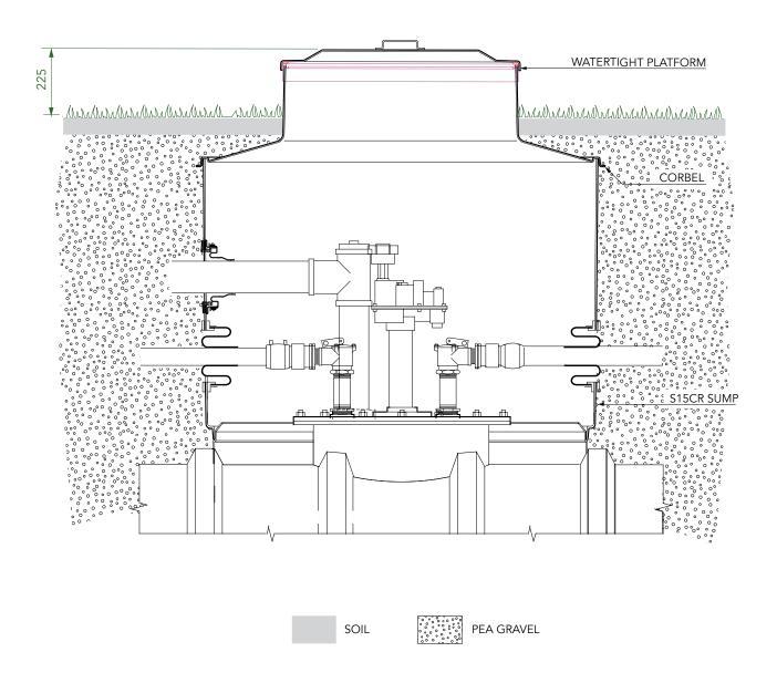
$1.45m\ diameter\ sump\ with\ collar\ ring,\ corbel\ and\ watertight\ platform.$  Designed for green area applications.
