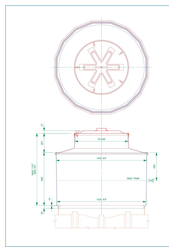
1.45m diameter sump with collar ring, corbel and watertight platform. Designed for green area applications.
