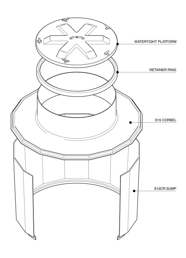
1.45m diameter sump with collar ring, corbel and watertight platform. Designed for green area applications.
