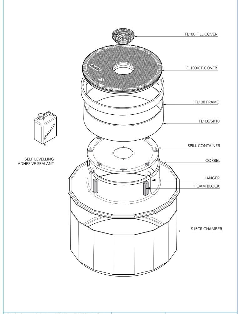
1.45m diameter sump with collar ring, corbel,platform, adjustable height skirt and round 1020mm flat sealed cover and frame with central fill cover.
