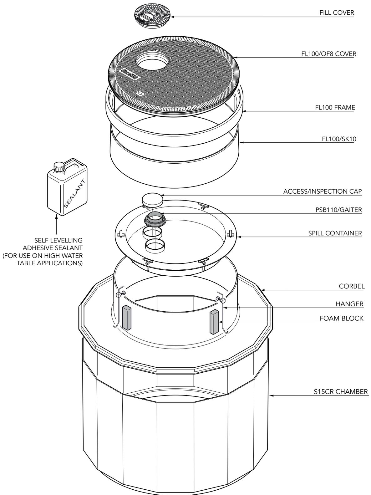
1.45m diameter sump with collar ring, corbel, adjustable height skirt, spill container with drainback Valve, and round 900mm flat sealed cover with offset fill cover and frame. Inc. PSB/110 Pipekit
