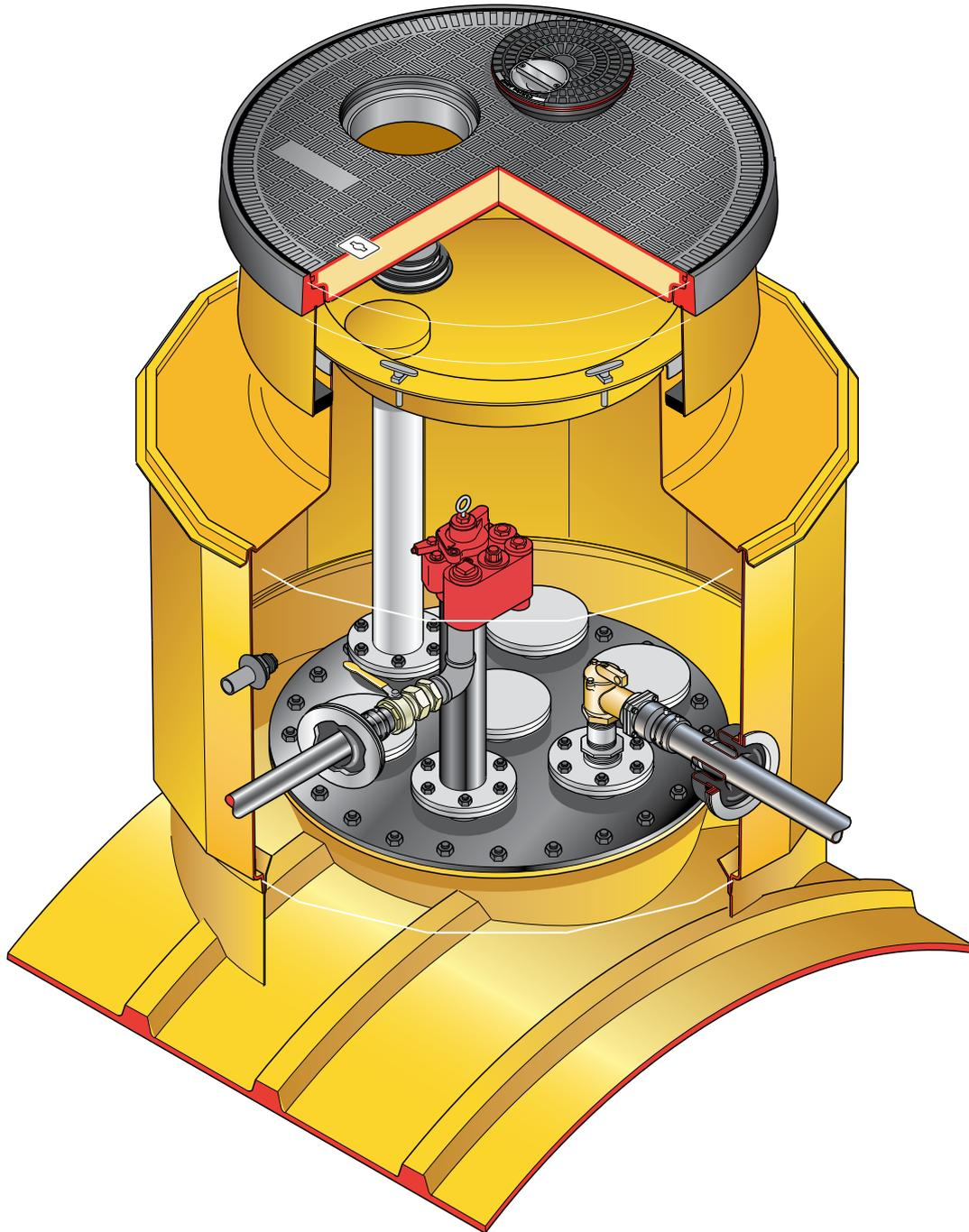
1.45m diameter sump with collar ring, corbel, adjustable height skirt, spill container with drainback Valve, and round 900mm flat sealed cover with offset fill cover and frame. Inc. PSB/110 Pipekit
