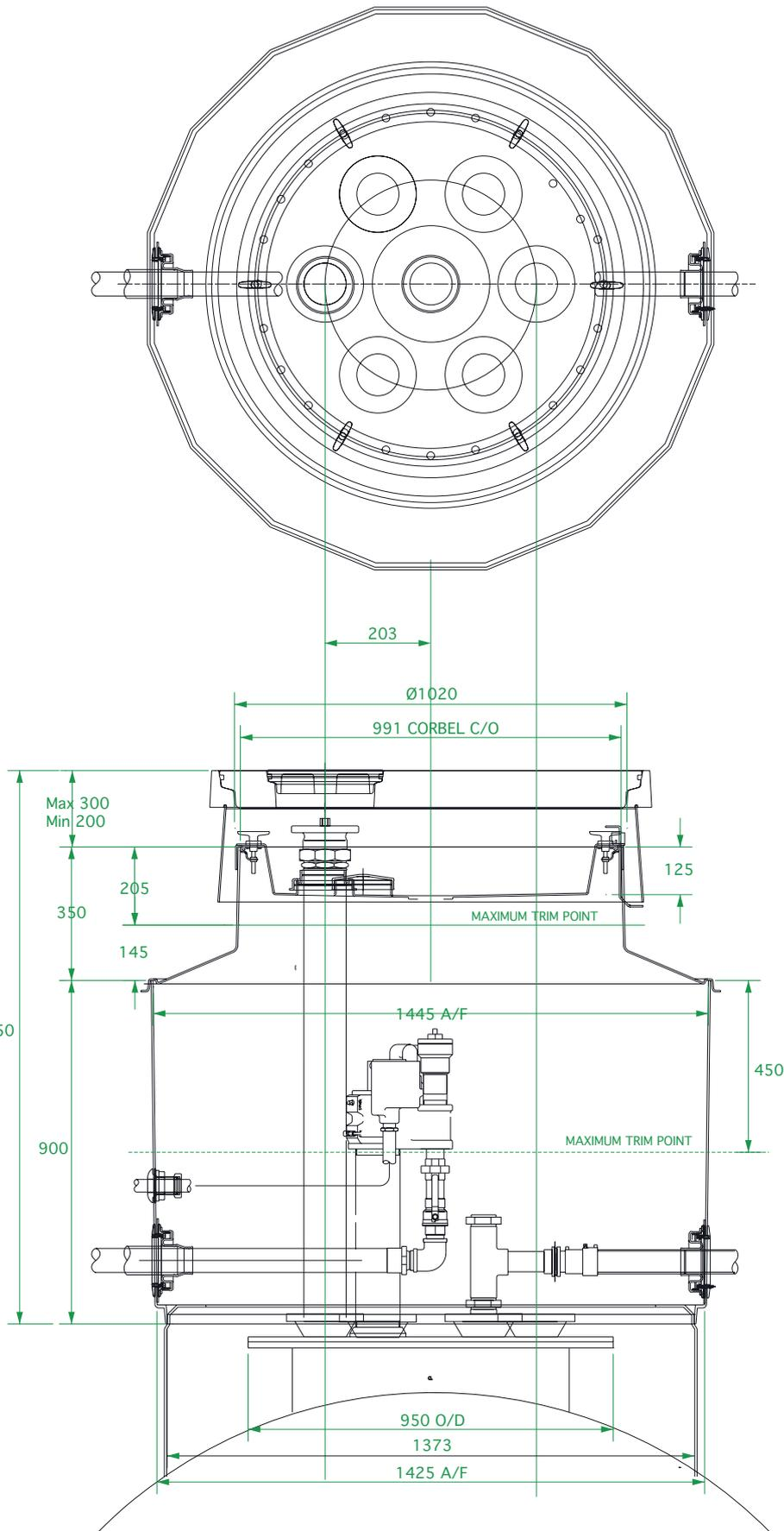
1.45m diameter sump with collar ring, corbel, adjustable height skirt, spill container with drainback Valve, and round 900mm flat sealed cover with offset fill cover and frame. Inc. PSB/110 Pipekit
