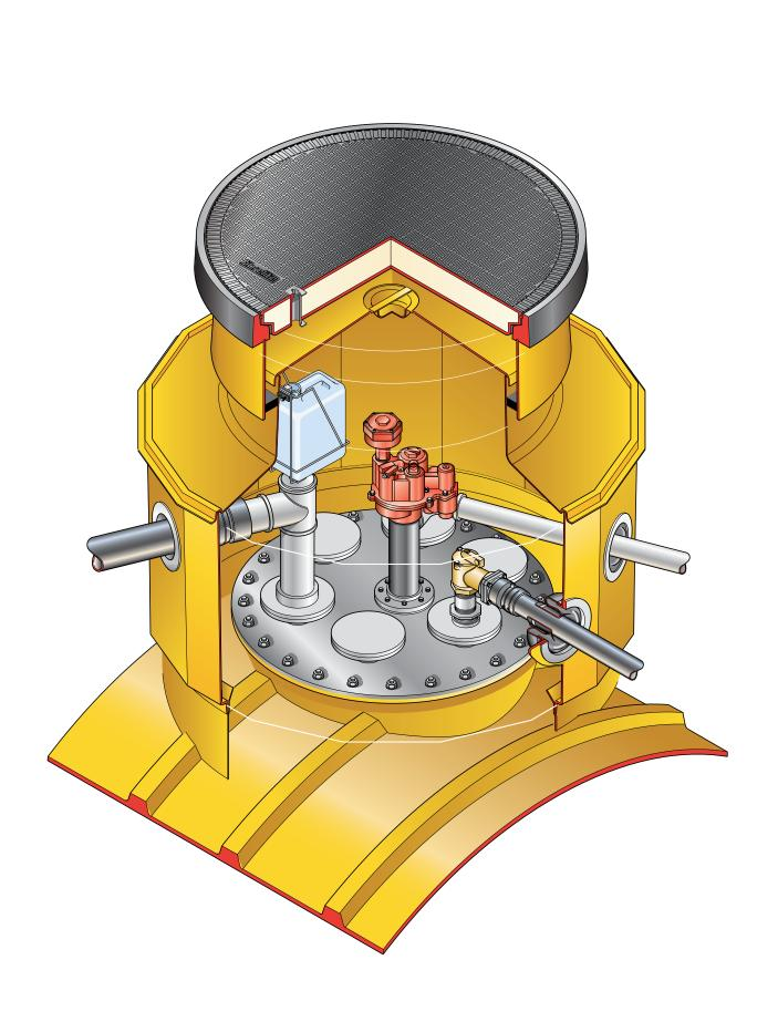
1.45 m diameter sump with collar ring, corbel, adjustable height skirt and round 1020mm flat sealed cover and frame.
