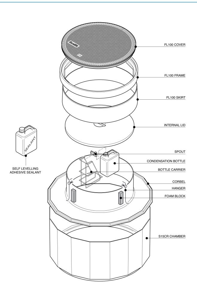
1.45 m diameter sump with collar ring, corbel, adjustable height skirt and round 1020mm flat sealed cover and frame.
