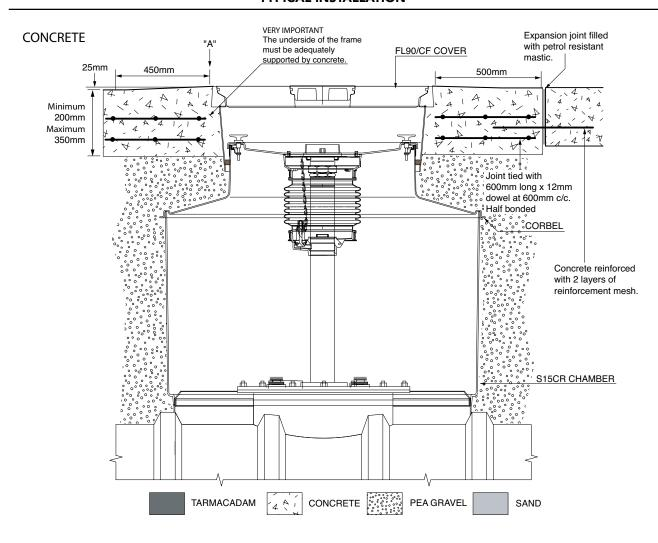
1.45m diameter sump with collar ring, corbel, spill platform to fit OPW spill bucket, adjustable height skirt and round 900mm flat sealed cover with central fill cover and frame. For reference purposes only. This drawing is not a specification. Order against product code only. To enable continuous improvement of our products, the designs and specifications are subject to change without notice.
