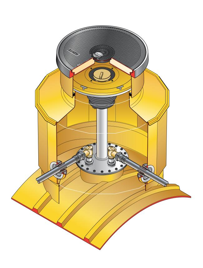
1.45m diameter sump with collar ring, corbel, spill platform to fit OPW spill bucket, adjustable height skirt and round 900mm flat sealed cover with central fill cover and frame.
