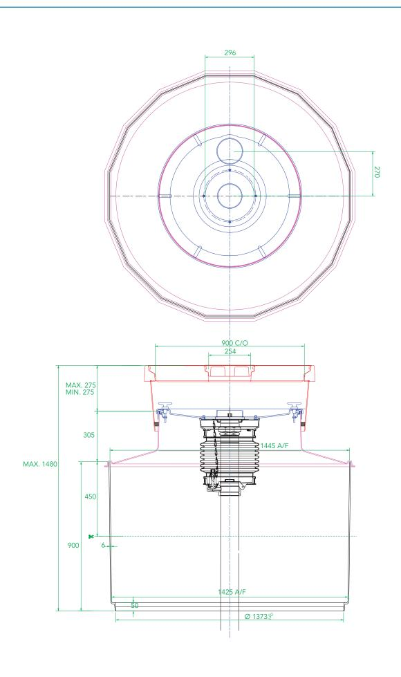
1.45m diameter sump with collar ring, corbel, spill platform to fit OPW spill bucket, adjustable height skirt and round 900mm flat sealed cover with central fill cover and frame.
