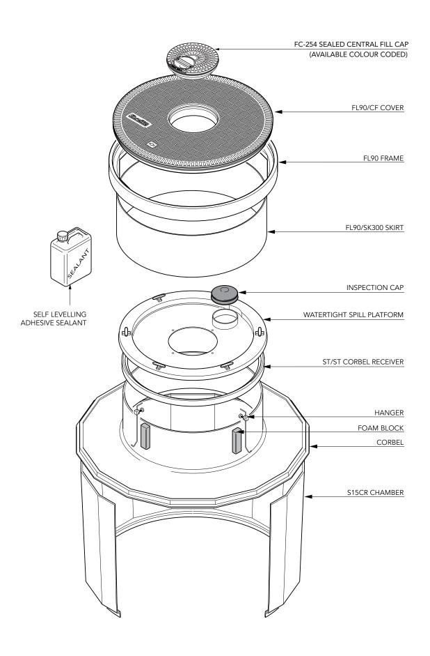
1.45m diameter sump with collar ring, corbel, spill platform to fit OPW spill bucket, adjustable height skirt and round 900mm flat sealed cover with central fill cover and frame. For reference purposes only. This drawing is not a specification. Order against product code only. To enable continuous improvement of our products, the designs and specifications are subject to change without notice.
