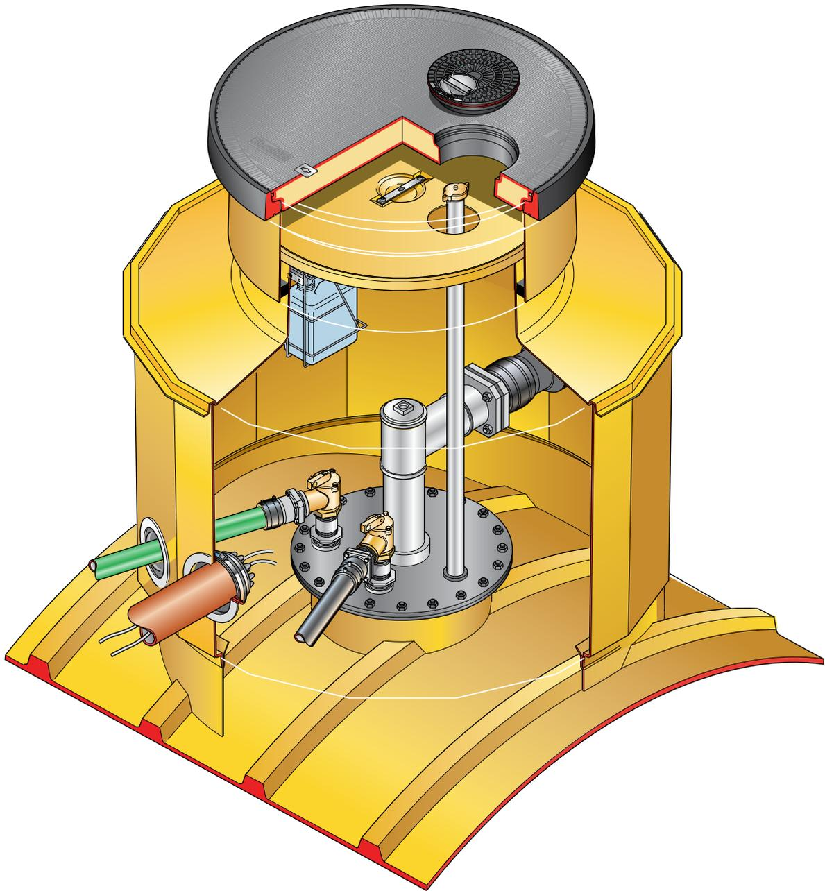
1.45m diameter sump with collar ring, corbel, internal lid, adjustable height skirt and round 900mm flat sealed cover with offset manual dip cover and frame.
