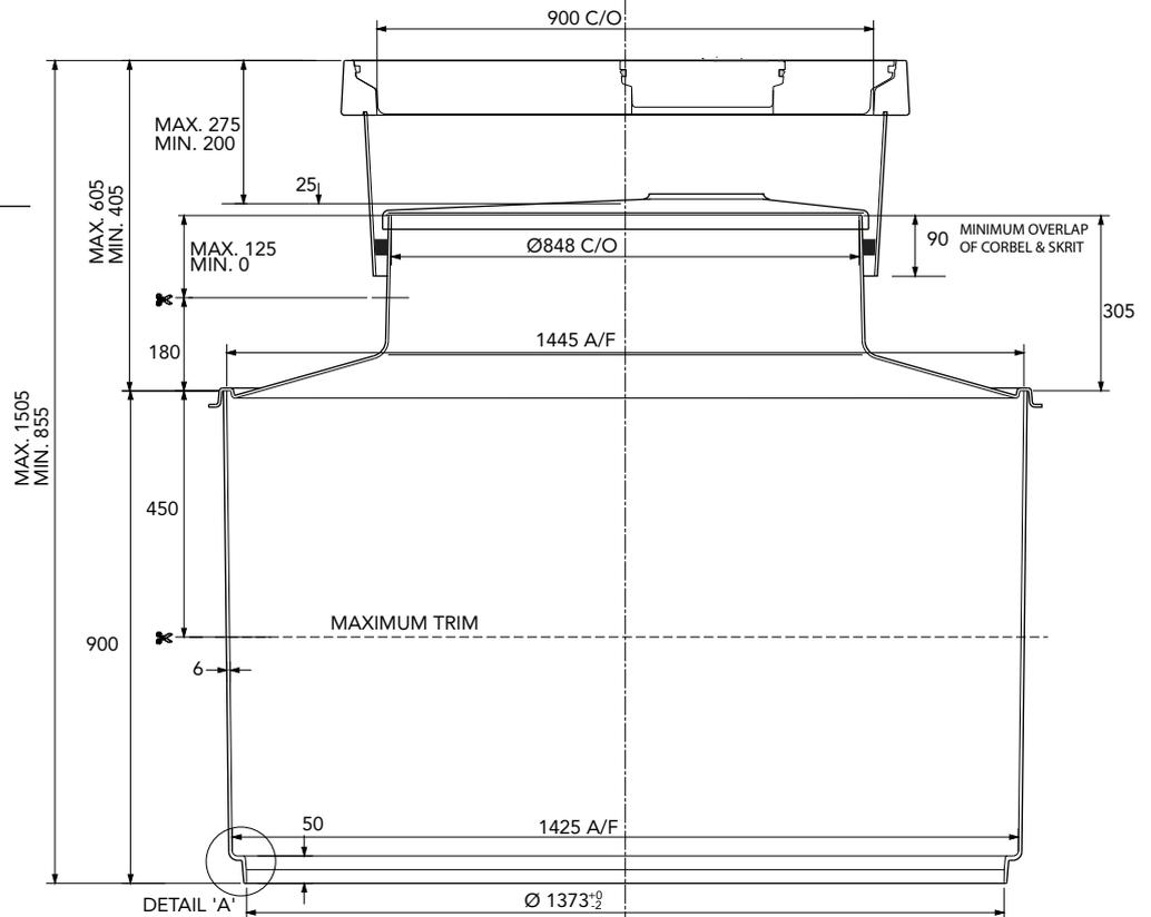
1.45m diameter sump with collar ring, corbel, internal lid, adjustable height skirt and round 900mm flat sealed cover with offset manual dip cover and frame.
