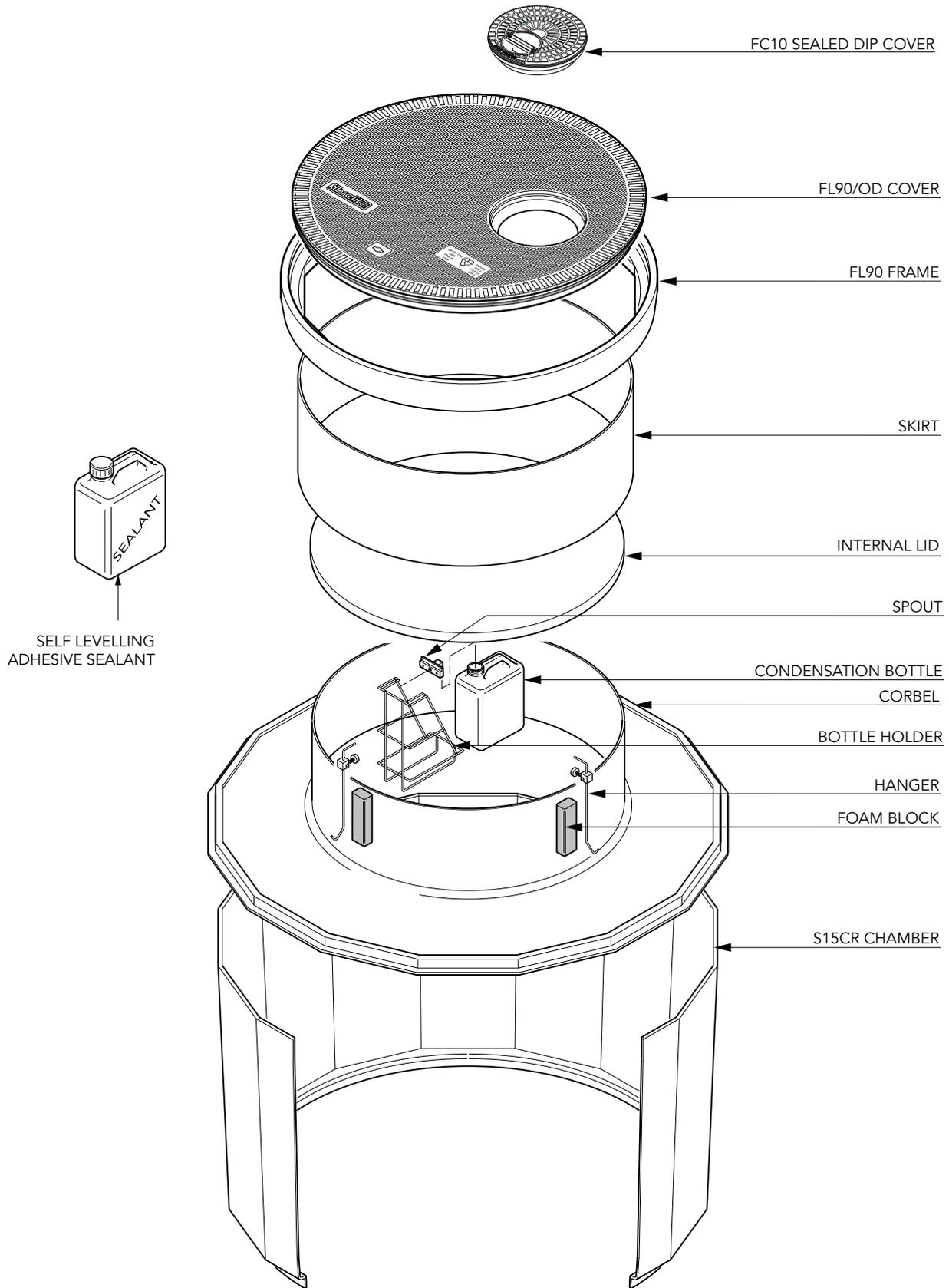
1.45m diameter sump with collar ring, corbel, internal lid, adjustable height skirt and round 900mm flat sealed cover with offset manual dip cover and frame.
