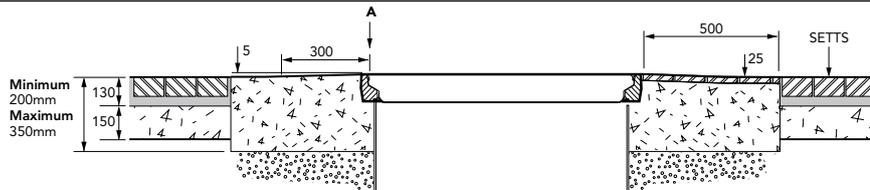
1.45m diameter sump with collar ring, corbel, internal lid, adjustable height skirt and round 900mm flat sealed cover with offset manual dip cover and frame.
