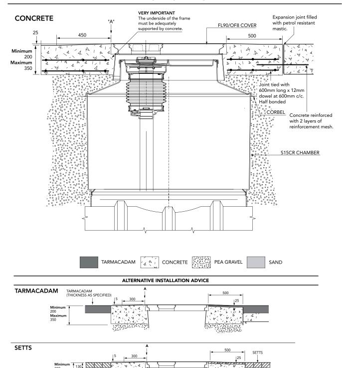
1.2m diameter bolted base chamber, corbel, internal lid with a height adjustable skirt and round 900mm flat sealed cover with a centre dip port. Includes sealkit with condensation bottle and fixing kit. Round tank flange. Remote Fill
