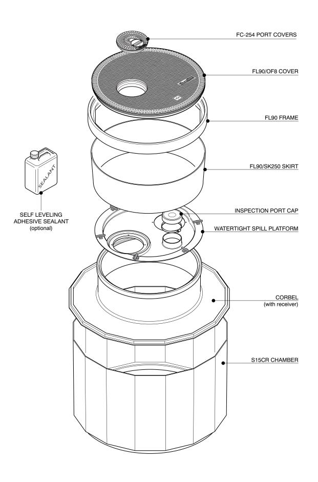
1.2m diameter bolted base chamber, corbel, internal lid with a height adjustable skirt and round 900mm flat sealed cover with a centre dip port. Includes sealkit with condensation bottle and fixing kit. Round tank flange. Remote Fill
