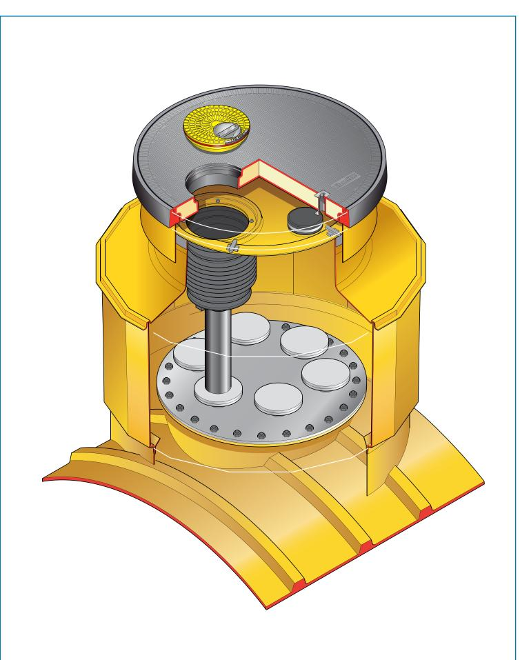
1.2m diameter bolted base chamber, corbel, internal lid with a height adjustable skirt and round 900mm flat sealed cover with a centre dip port. Includes sealkit with condensation bottle and fixing kit. Round tank flange. Remote Fill
