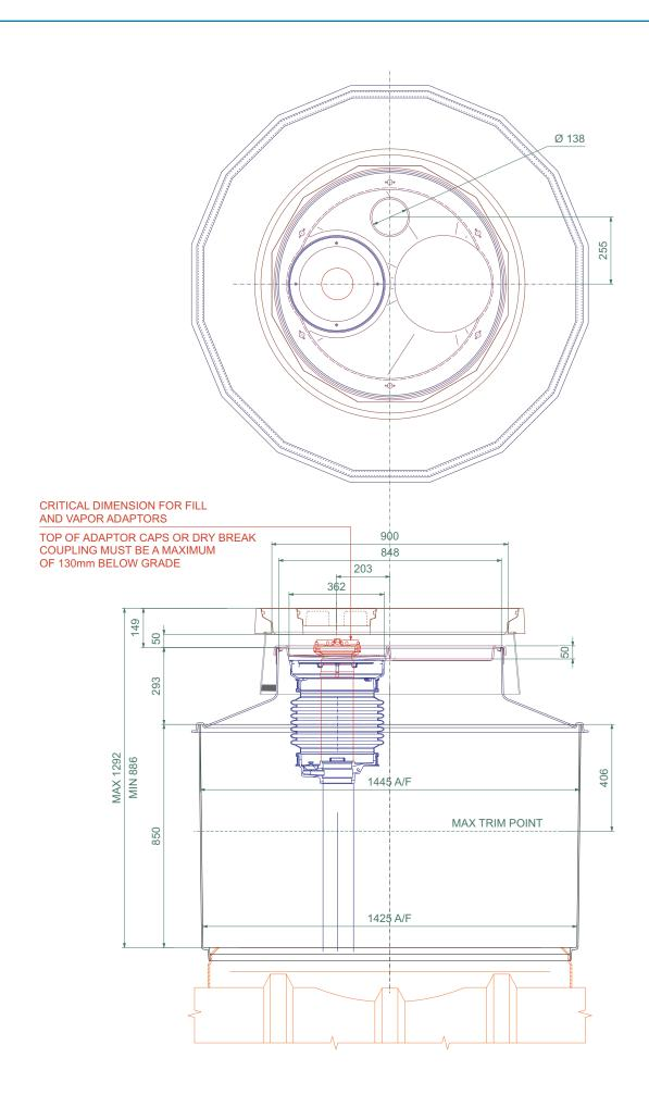
1.2m diameter bolted base chamber, corbel, internal lid with a height adjustable skirt and round 900mm flat sealed cover with a centre dip port. Includes sealkit with condensation bottle and fixing kit. Round tank flange. Remote Fill
