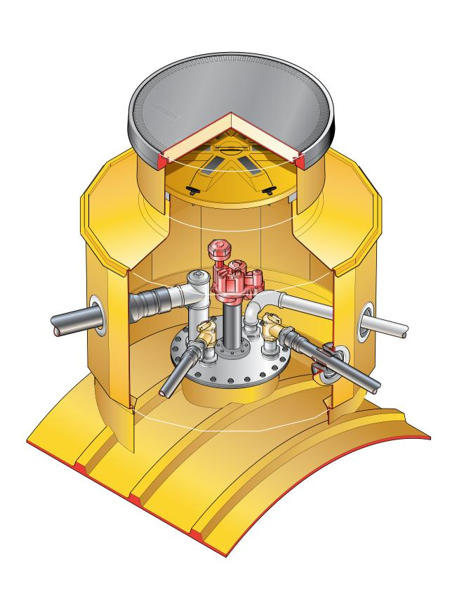
$1.45 m\ diameter\ sump\ with\ collar\ ring,\ corbel,\ sealed\ watertight\ lid,\ adjustable\ height\ skirt\ and\ round\ 900 mm\ flat\ sealed\ cover\ and\ frame.$
