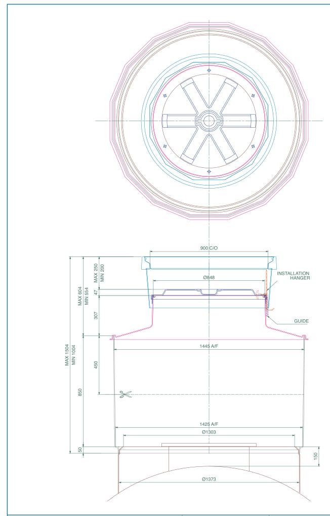
1.45m diameter sump with collar ring, corbel, sealed watertight lid, adjustable height skirt and round 900mm flat sealed cover and frame.
