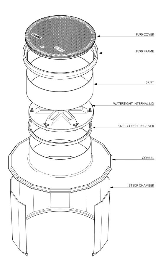
$1.45 m\ diameter\ sump\ with\ collar\ ring,\ corbel,\ sealed\ watertight\ lid,\ adjustable\ height\ skirt\ and\ round\ 900 mm\ flat\ sealed\ cover\ and\ frame.$
