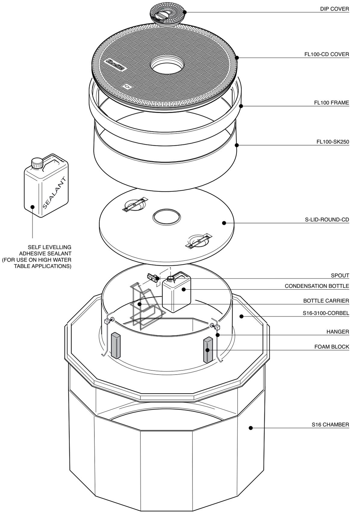
1.5m diameter 12 sided sump with reverse flange, corbel, adjustable height skirt, internal lid with dip tube hole, and round 1020mm flat sealed cover and frame with central dip cover.
