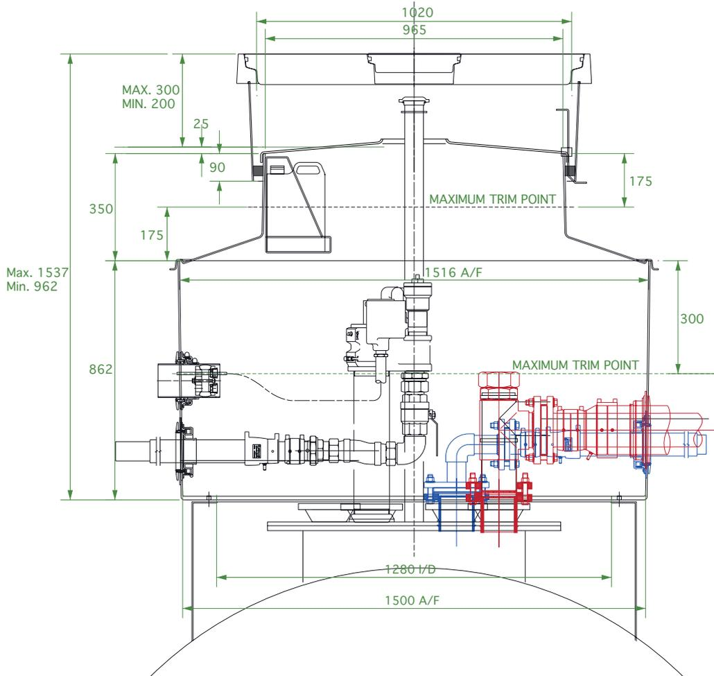
1.5m diameter 12 sided sump with reverse flange, corbel, adjustable height skirt, internal lid with dip tube hole, and round 1020mm flat sealed cover and frame with central dip cover.
