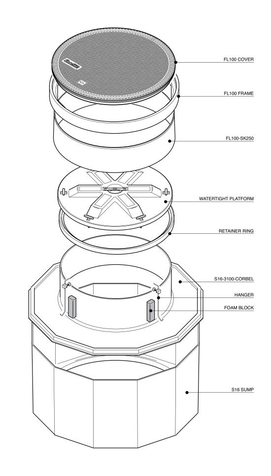
1.5m diameter 12 sided sump with reverse flange, corbel, adjustable height skirt, internal watertight platform, round 1020mm flat sealed cover and frame. Beild continuous improvement of our products, the designs and specifications are subject to change without notice.
