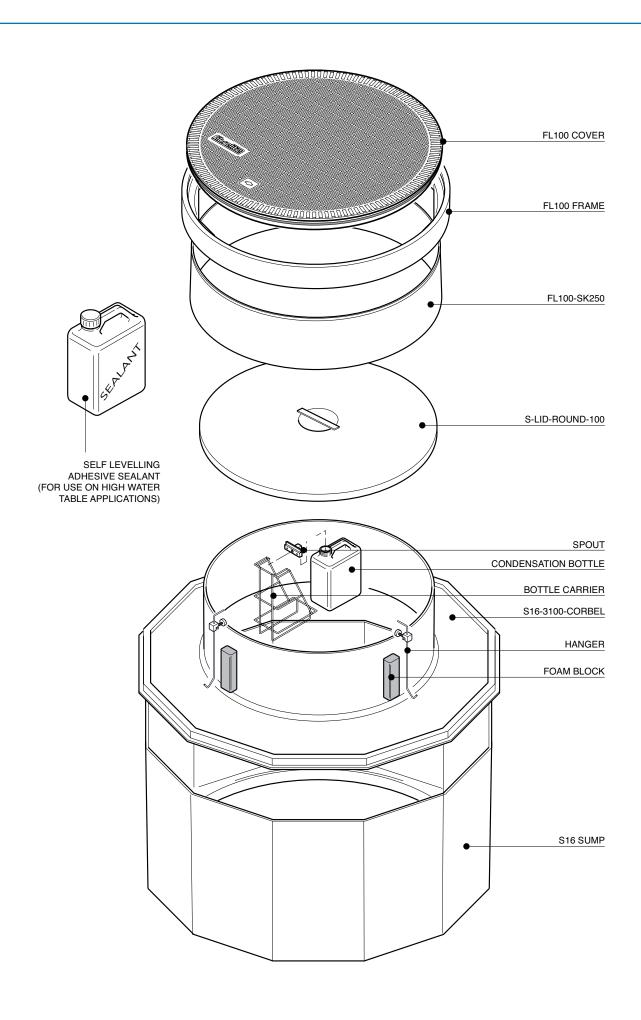
1.5 m diameter 12 sided sump with reverse flange, corbel, adjustable height skirt, internal lid, and round 1020mm flat sealed cover and frame.
