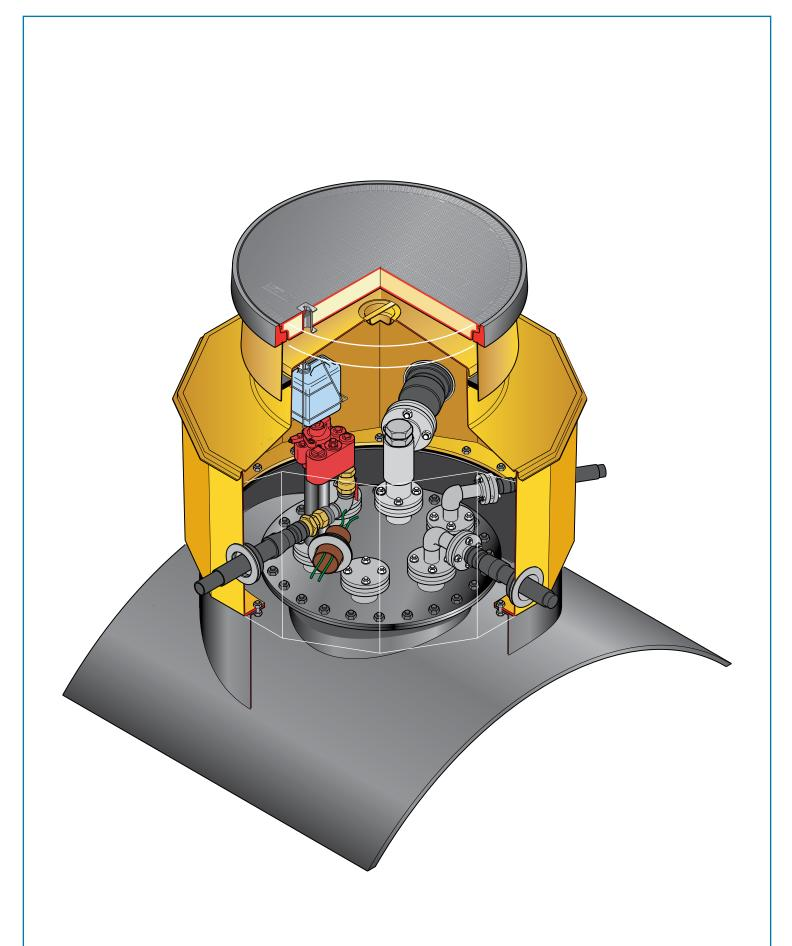
1.5 m diameter 12 sided sump with reverse flange, corbel, adjustable height skirt, internal lid, and round 1020mm flat sealed cover and frame.
