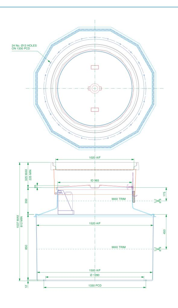
1.5 m diameter 12 sided sump with reverse flange, corbel, adjustable height skirt, internal lid, and round 1020mm flat sealed cover and frame.
